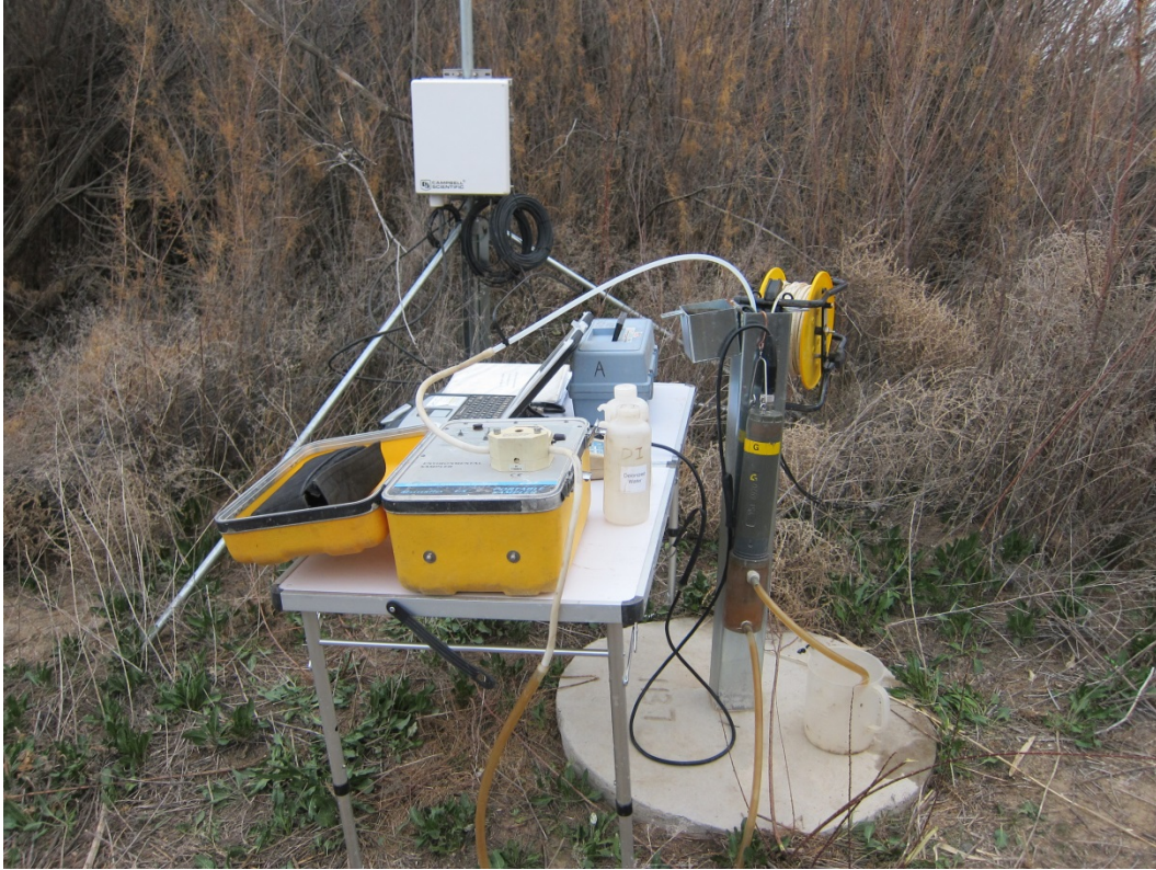
Figure 3: Groundwater sampling at well with telemetry device in floodplain
