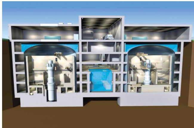
Conceptual drawing of an underground containment structure housing two B&W mPower reactor modules.
