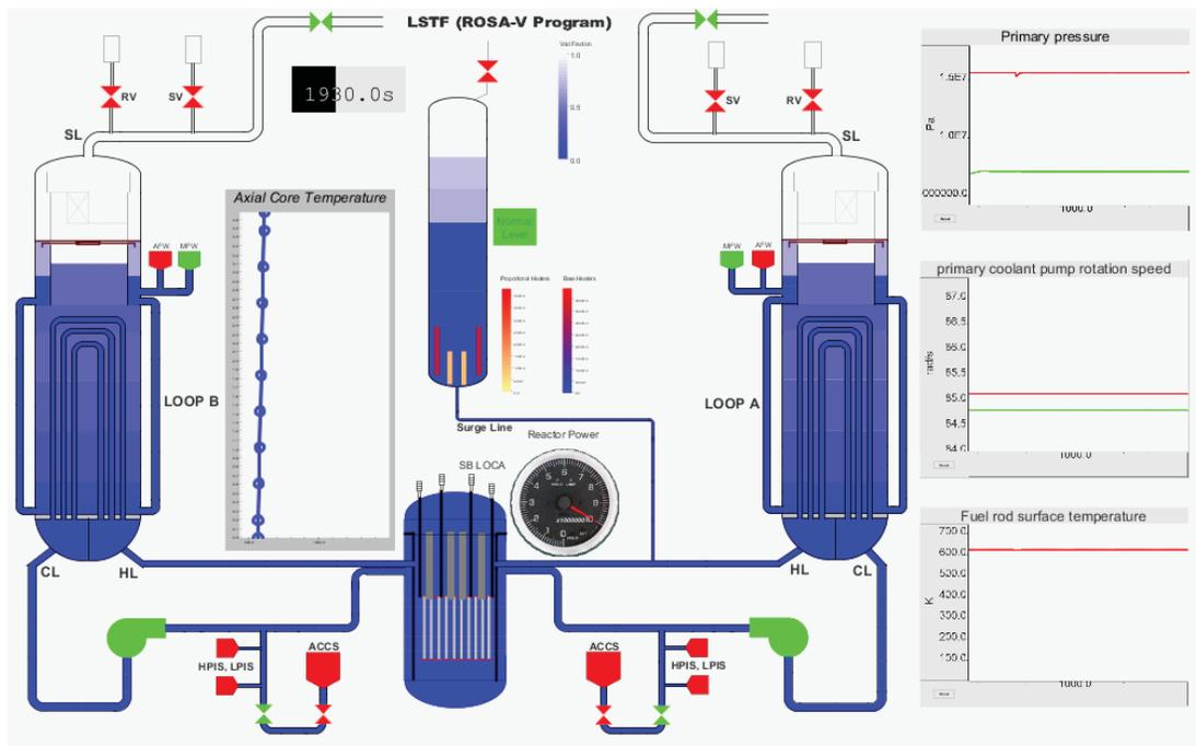
Figure 10: SNAP mask for LSTF TRACE model
