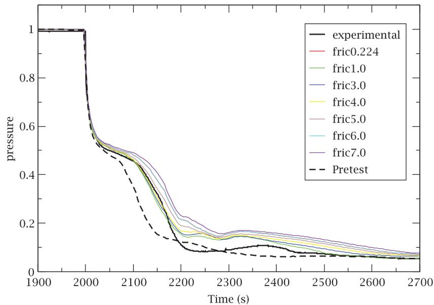
Figure 15: Normalized primary pressure. Friction factor sensitivity
