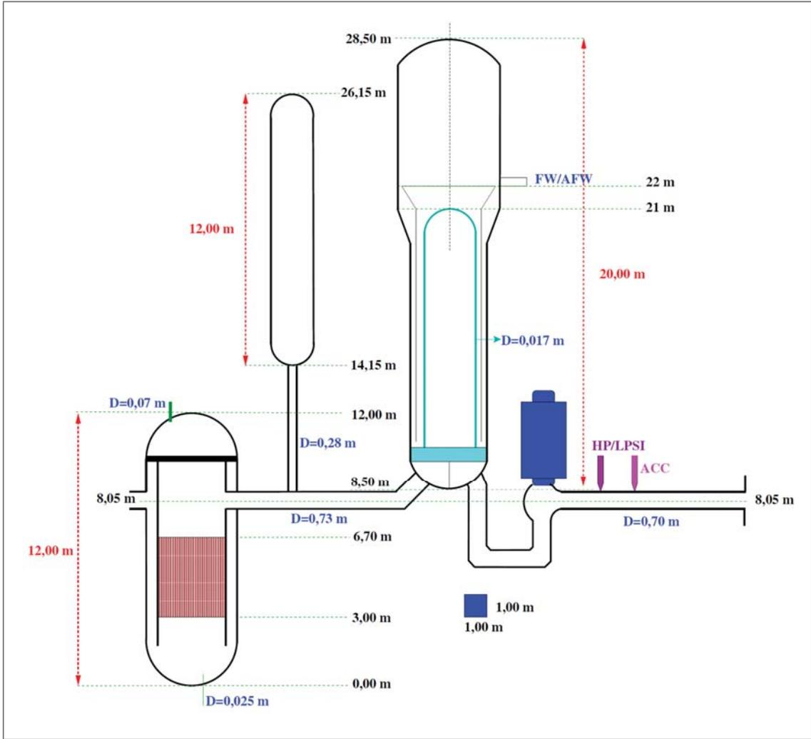
Figure 27: Scheme of Almaraz NPP (elevation view)
