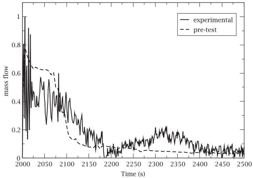
Figure 13: Discharge mass flow. Experimental and pre-test simulation
