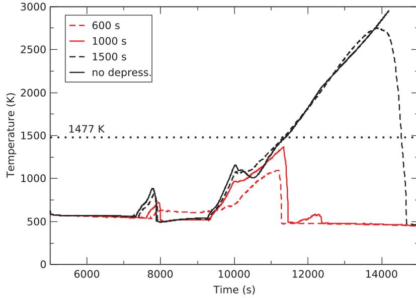
Figure 35: PCT. Sensitivity to SG depressurization. Break diameter: 2".
