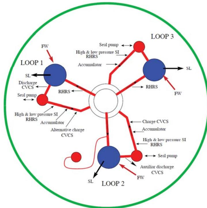
Figure 26: Scheme of Almaraz NPP (plan view)
