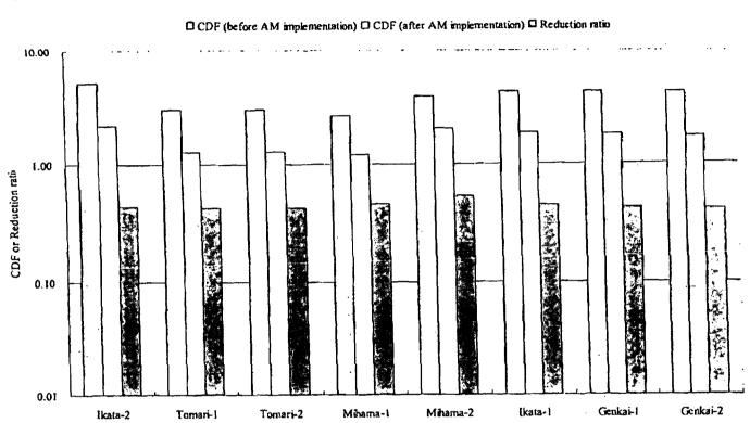
Another example can be find in type A group. ECCS switch-over from the injection mode to the recirculation mode is done automatically for Tomari-1 and 2, while this operation is done by operator for other NPPs of type A group. This design difference makes CDFs of Tomari-1 and 2 smaller than CDFs of the other plants in type A group.
