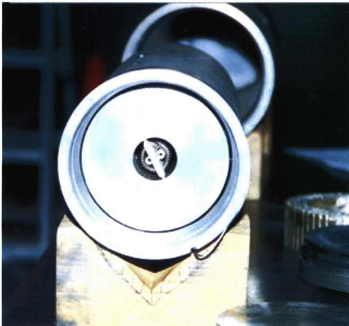
Figure 2 Photograph of the heater and replicate mass used in the Sandia test.
