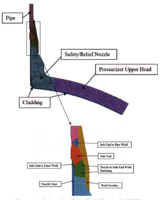
Figure 4-1: Schematic of Safety/Relief Nozzle with FSWOL
