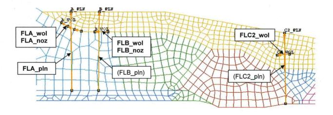
Figure 4-8: PZR Safety Nozzle with Path Lines Superposed
