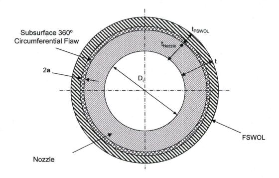
Figure 2-3: PZR Safety Nozzle A Idealized Indication
