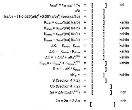
The calculated 2a = [ ] inch is the initial 2a for the next transient crack growth calculation. After going through all 10 transients in the first year, the crack grows from [ ], which confirms the results obtained in Table 7-2 for the first year. Then, [ ] is used as the initial crack length for the second year calculation and so on. Thus by repeating the process the final flaw size at the end of 38 years is obtained.
