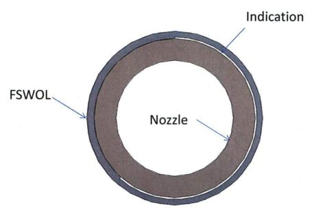
Figure 2-2: Planar Projection of PZR Safety Nozzle A Indication
