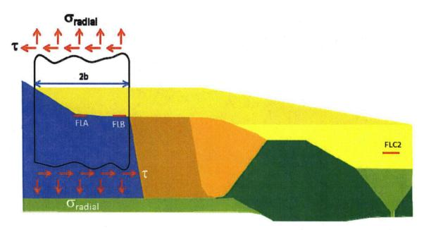
Notes: 1) For laminar indications represented by Flaw FLA (indications - #1, #1A in Nozzle A, Indication #3 in Nozzle C) and FLB (Indication #1, #2 and #3 in Nozzle B) the 2b parameter was defined as the distance between the point where the overlay meets the nozzle on one end and the butter on the other end. This distance is estimated as 1.31".
