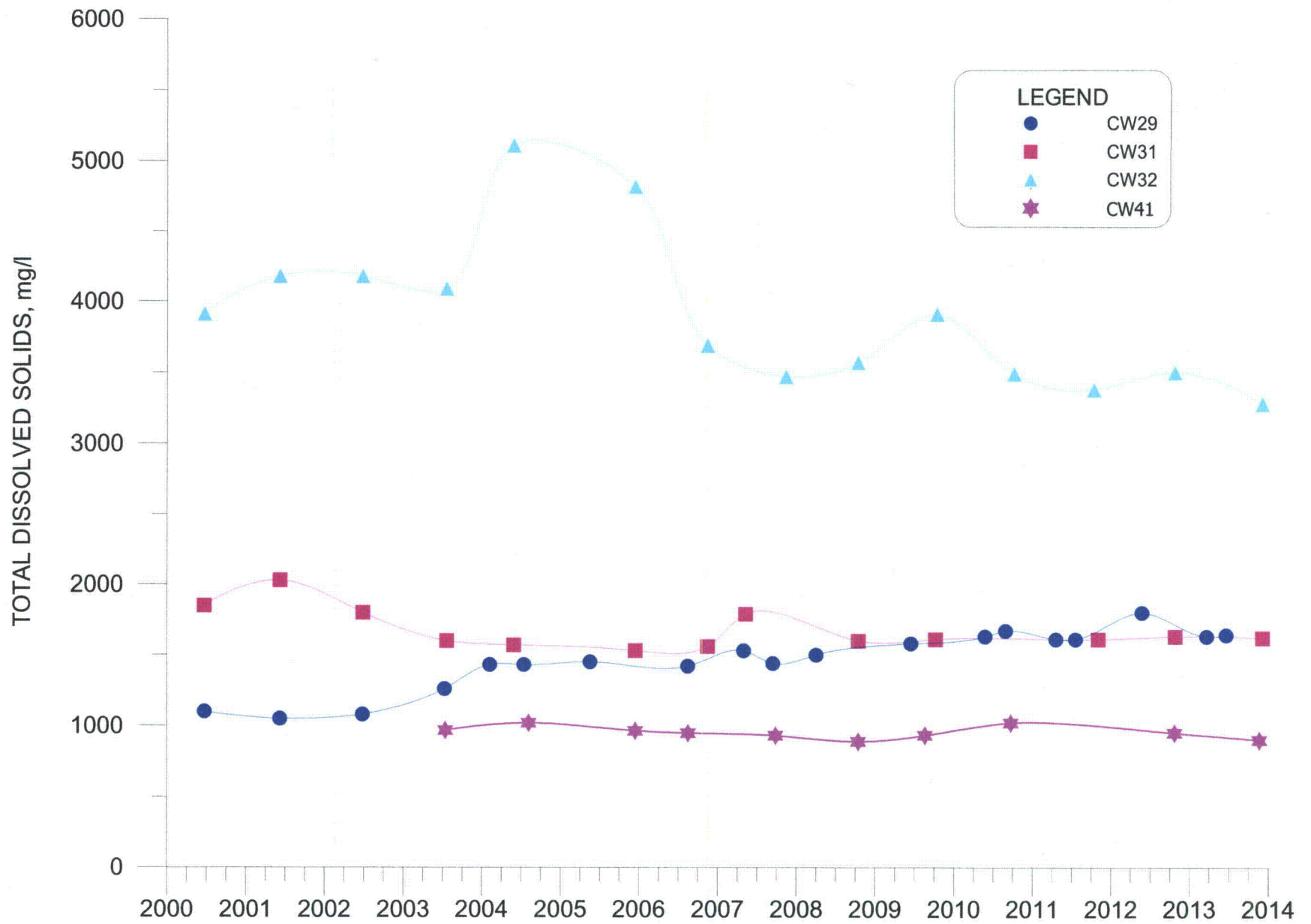
FIGURE 7.3-7. TDS CONCENTRATIONS FOR NON-MIXING ZONE WELLS CW29, CW31, CW32 AND CW41.
