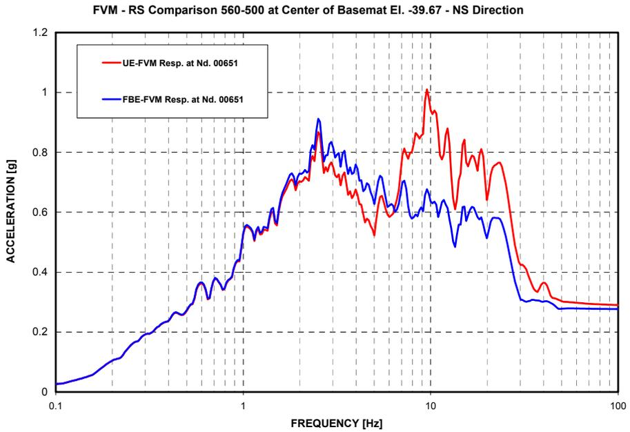
Figure 7 5% Damping ARS at Center, Basemat Bottom (el.-39.667 ft), NS Direction, FVM, 560-500 Soil
