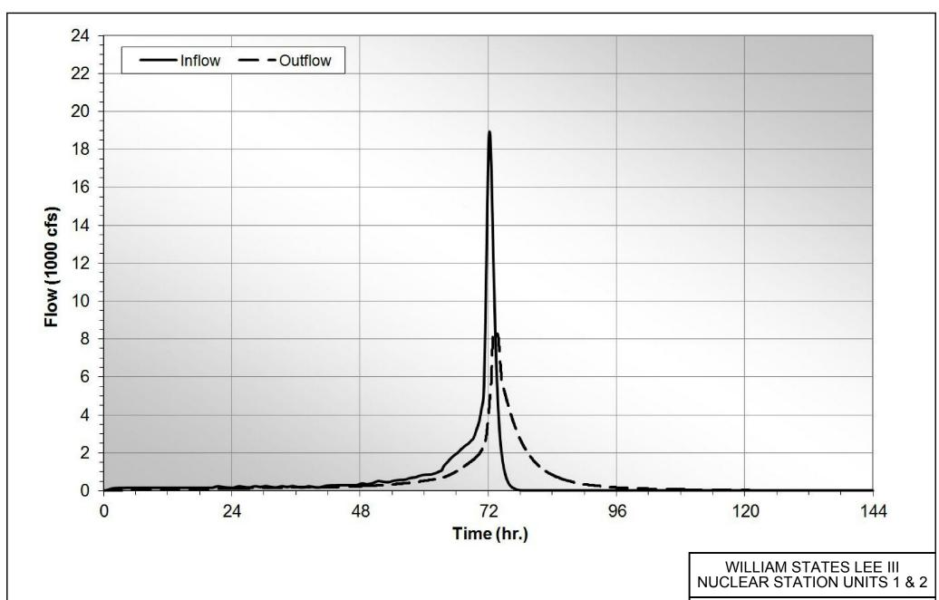
PMF Hydrograph Without Upper Arm Dam Failure, Make-Up Pond B
