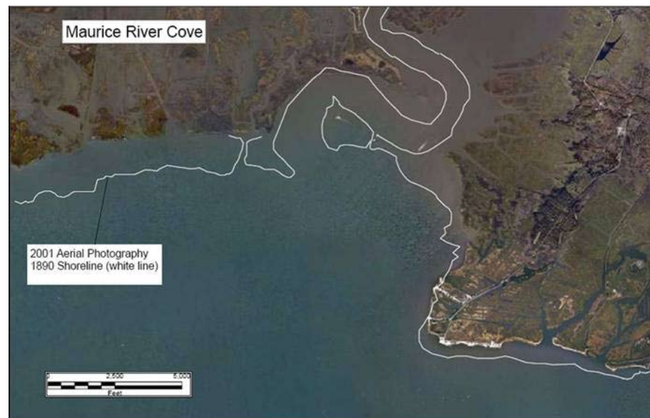
Fig. 1.21. Aerial Photo of Maurice River Cove comparing 2001 shoreline to that of 1890. Photo courtesy of J. Gebert, U.S. Army Corps of Engineers, Philadelphia District
