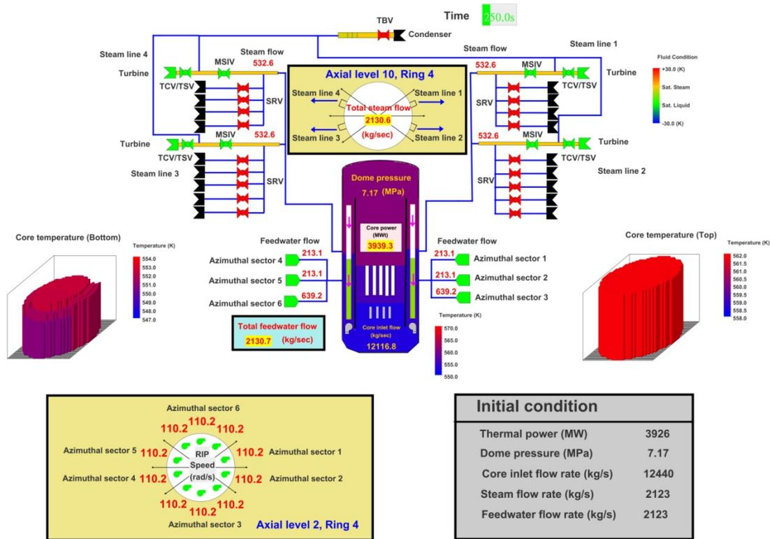
Figure 5 The initial condition and animation model of Lungmen
