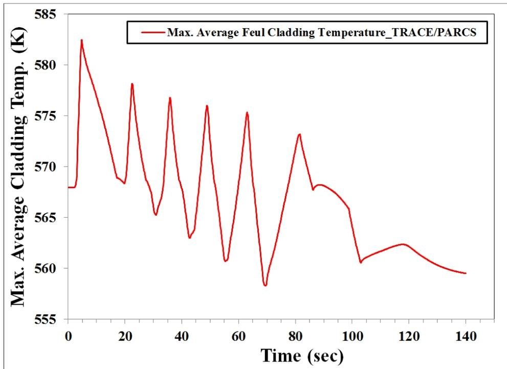
Figure 15 The maximum average cladding temperature (FMCRD run-in)
