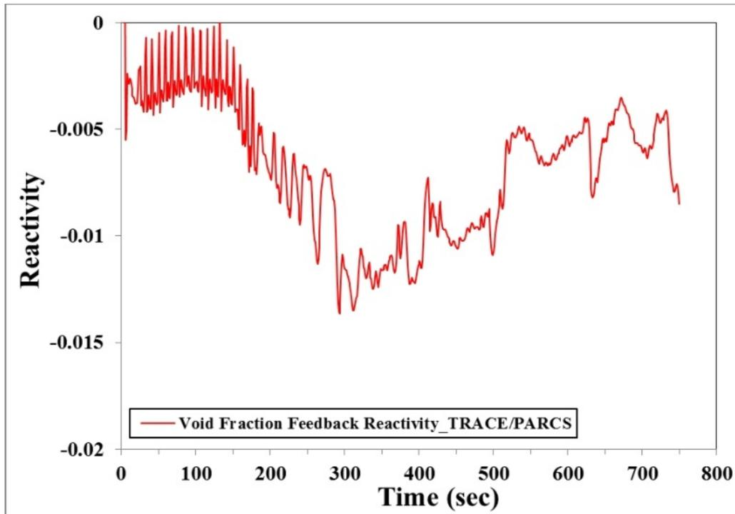
Figure 19 The void fraction feedback reactivity (SLCS initiation)
