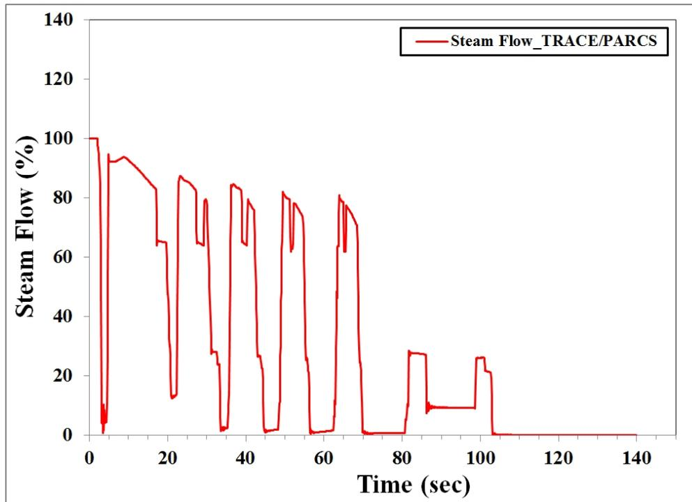
Figure 13 The steam flow (FMCRD run-in)
