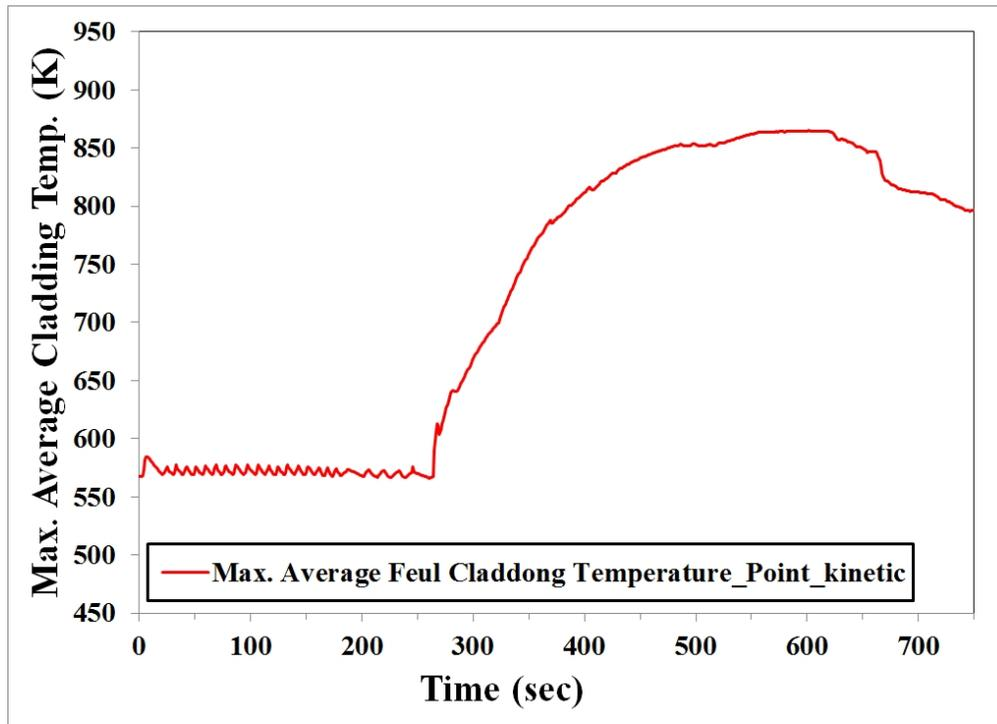
Figure 22 The maximum average cladding temperature (SLCS initiation)
