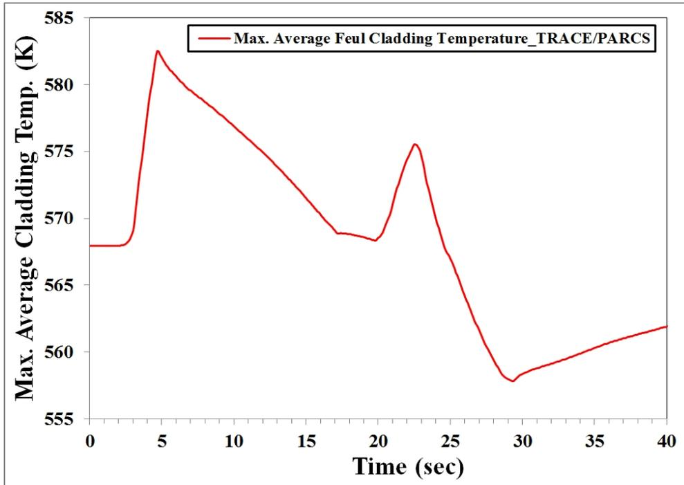
Figure 10 The maximum average cladding temperature (ARI)
