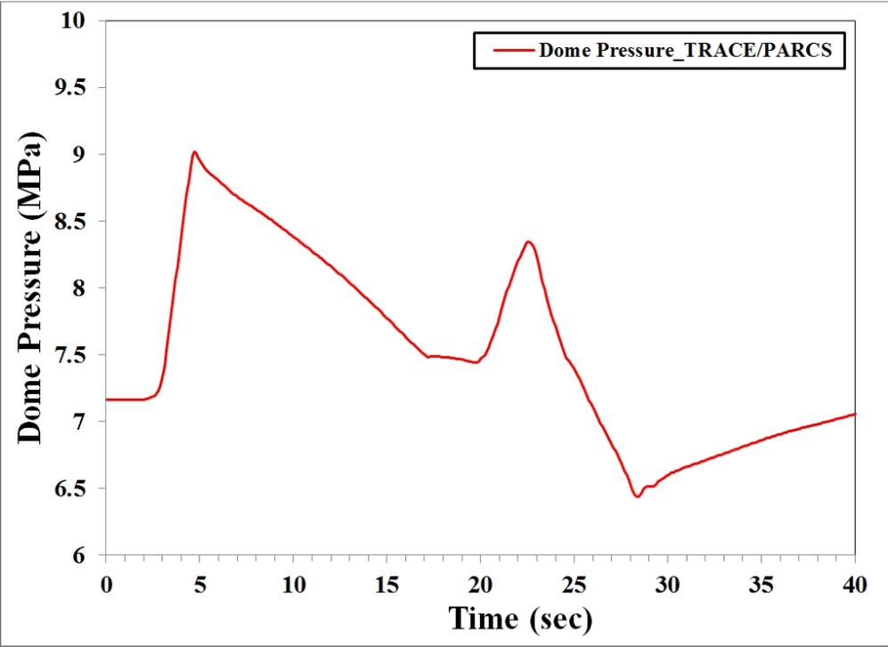
Figure 7 The dome pressure (ARI)
