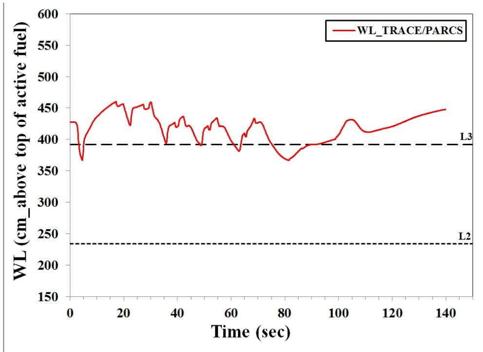
Figure 14 The water level (FMCRD run-in)
