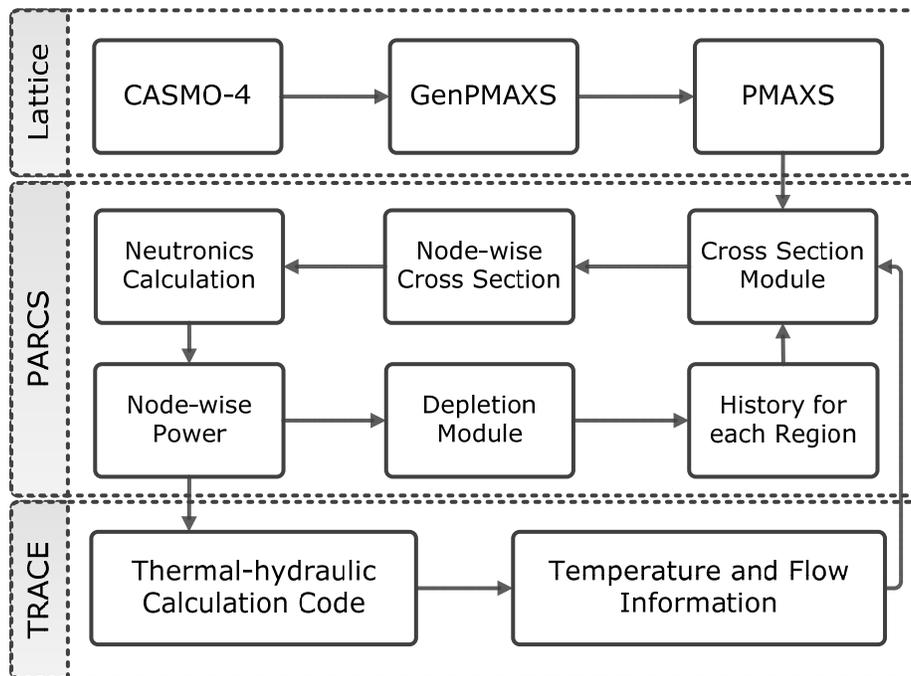
Figure 4 The procedure of TRACE/PARCS coupling calculation [4]
