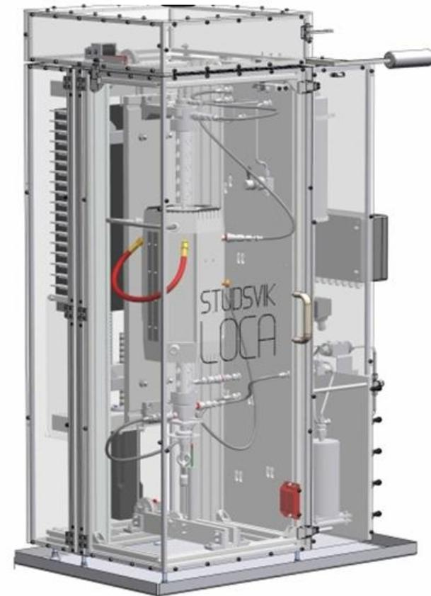
Conceptual design of new LOCA apparatus
