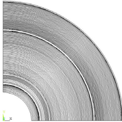
Figure A-7: Crack Front Propagation, Top View, Far Crack Case
