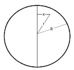
where the mean velocity is calculated by 1/X where x= X at r = R and V(x) is determined from the assumed V(r) where the relationship between x and r is obtained from the geometry illustrated in the figure.
