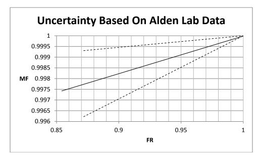
MF = 1 except at FR = 1 in contrast to the Caldon extrapolation of the data to the Caldon calculation that Caldon used to evaluate MF sensitivity. Further note that Caldon's approach results in a reduction in MF with increasing FR whereas the Alden data establishes that MF increases with increasing FR. In contrast, the absolute magnitude of the MF changes is identical due to the mirror image of the two calculations with respect to MF = 1.
