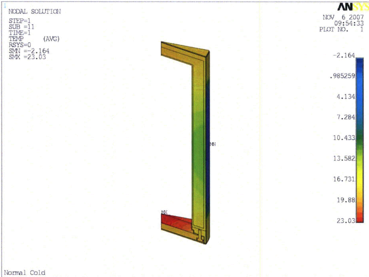
Figure 3-7 - Temperature Distribution – Normal Cold
