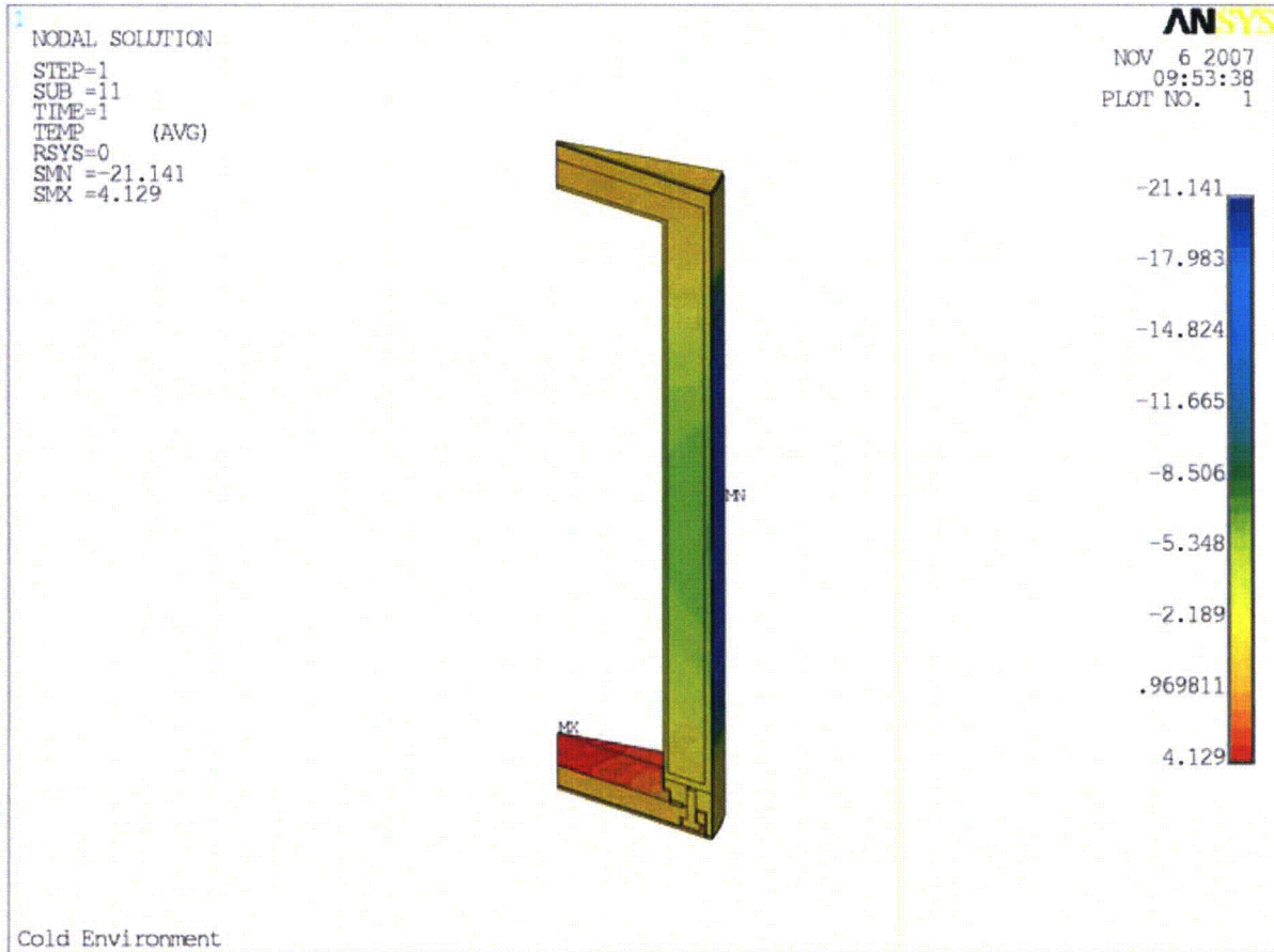
Figure 3-5 - Temperature Distribution – Cold Environment
