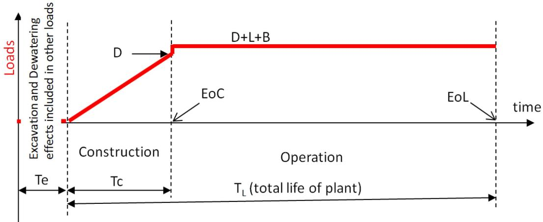
**Figure 1. Timeline of Loading for Settlement Analysis. Notations: D = Dead Loads, L = Live Loads, B = Loads from Backfill.**
