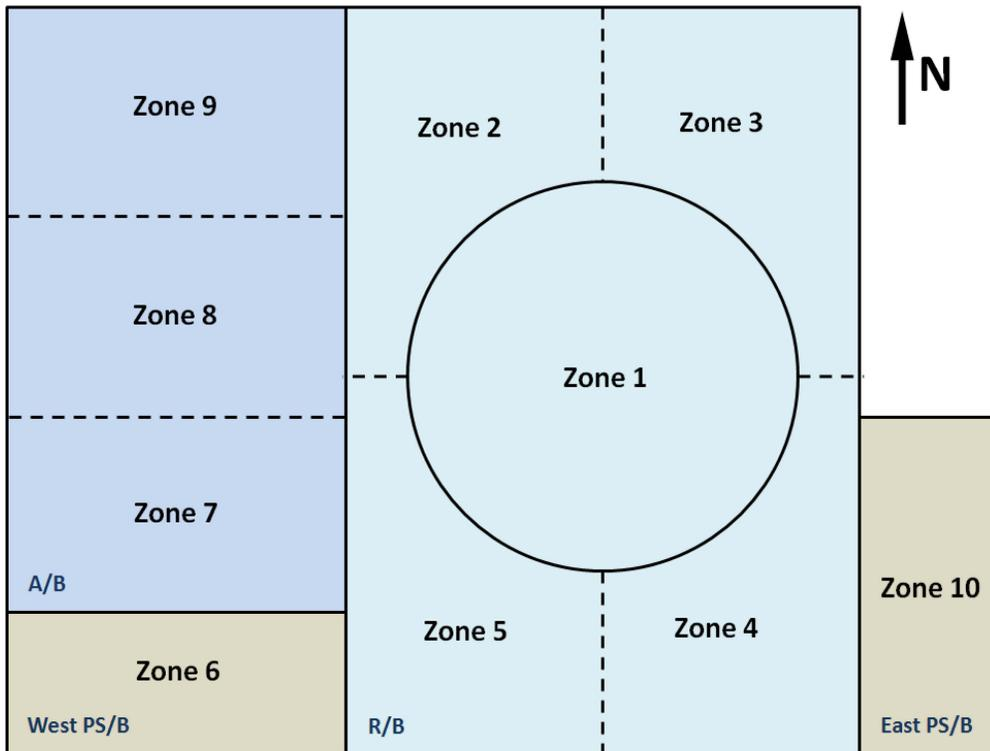
**Figure 3. Example of Basemat Concrete Placement Zones (Sequences) between Elevations -33'-0" and -26'-4" (Zone Numbering corresponds to Sequentially Outward Construction)**
