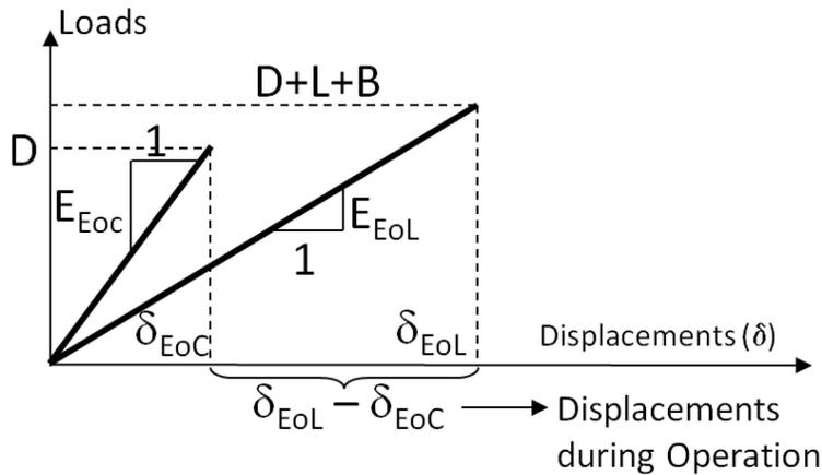
**Figure 2. Secant Moduli for Settlement Analysis**
