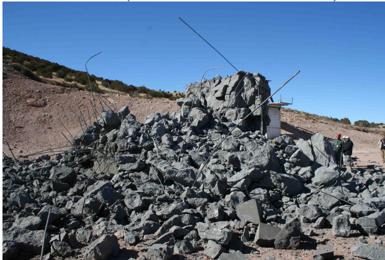
After Test (viewed from the attacked face)
