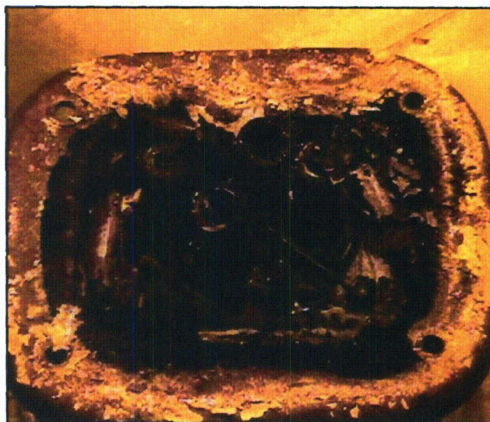
TP80(B) Thermal Test After Removal From Oven—Lid Removed
