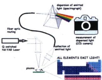
The technique utilizes a terawatt laser with nanosecond to femtosecond pulse durations to vaporize a minute amount of a target, about the target is analyzed using an optical emission spectrometry to determine the elemental and isotopic composition of the materials and contaminates present.
