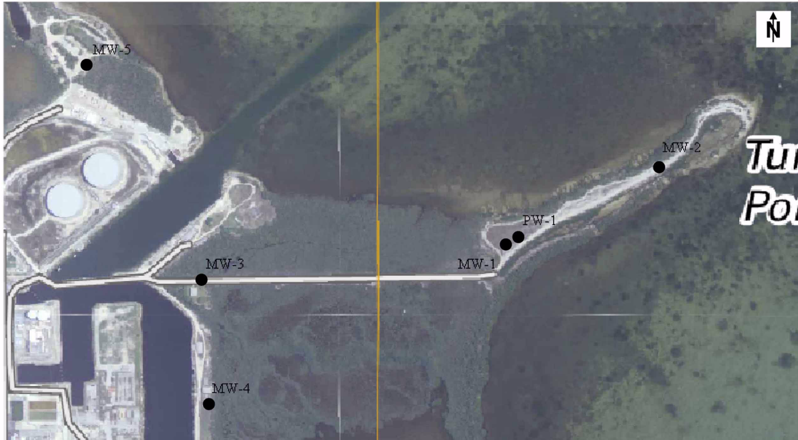
Figure 2.3-76 Layout of Pumping Test PW-1
