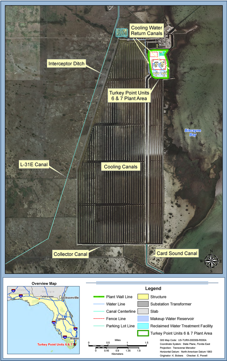
Figure 2.3-61 Industrial Wastewater Facility
