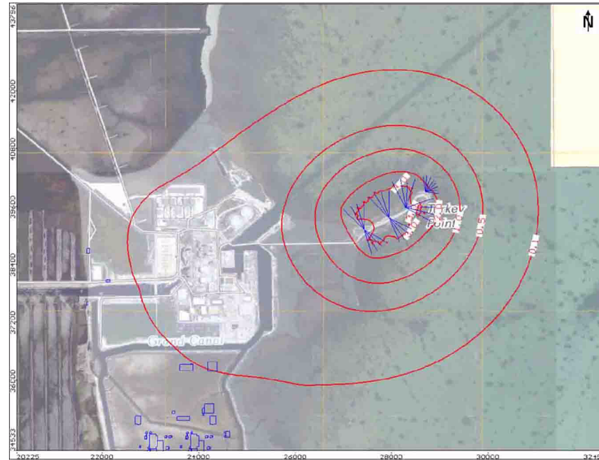
Figure 2CC-247 RCW Drawdown within the Pumped Layer (Upper Higher Flow Zone)
