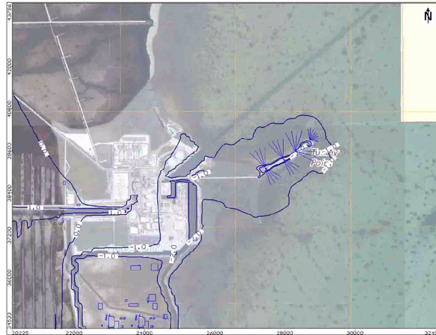
Figure 2CC-244 Head Contours in Layer 1 during Radial Collector Well Simulations
