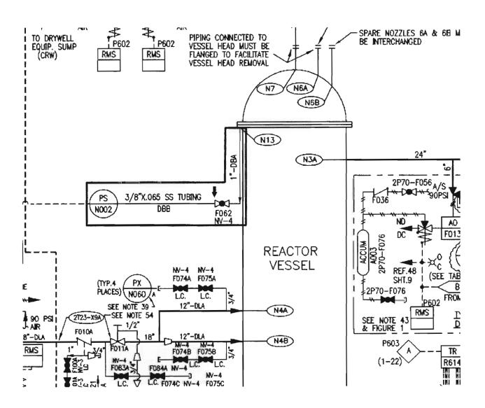
ATTACHMENT 3 Excerpt from Hatch Unit 2 P&ID H26000
