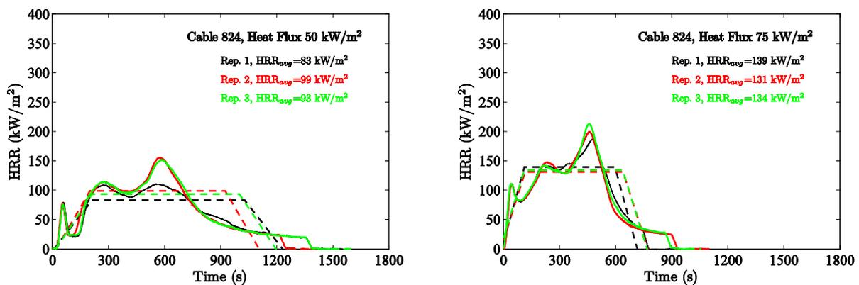
Figure 4-51. Results of cone calorimeter experiments, Cable 824.
