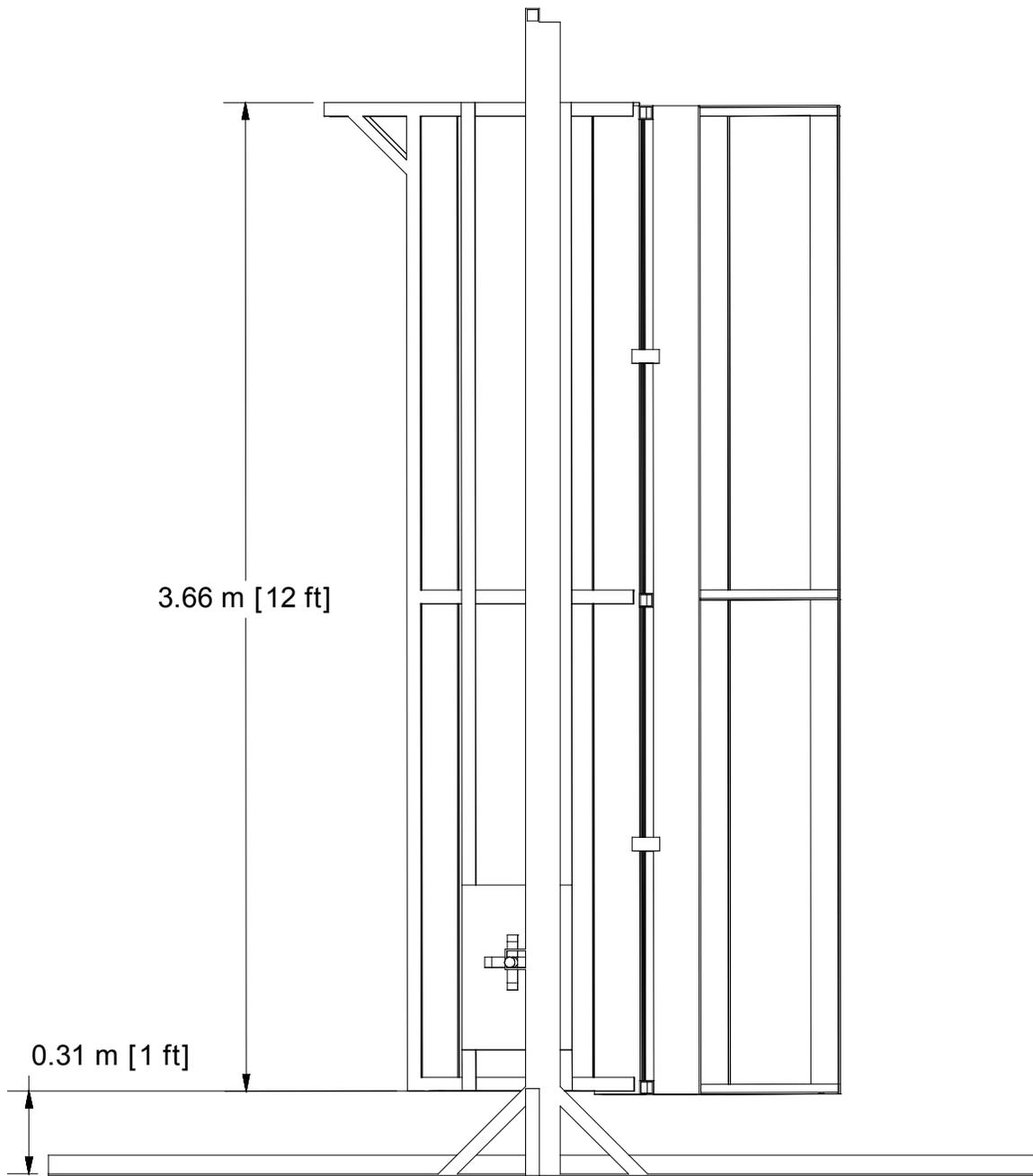
**Figure 5-1. Side view of the Vertical Tray Apparatus.**
