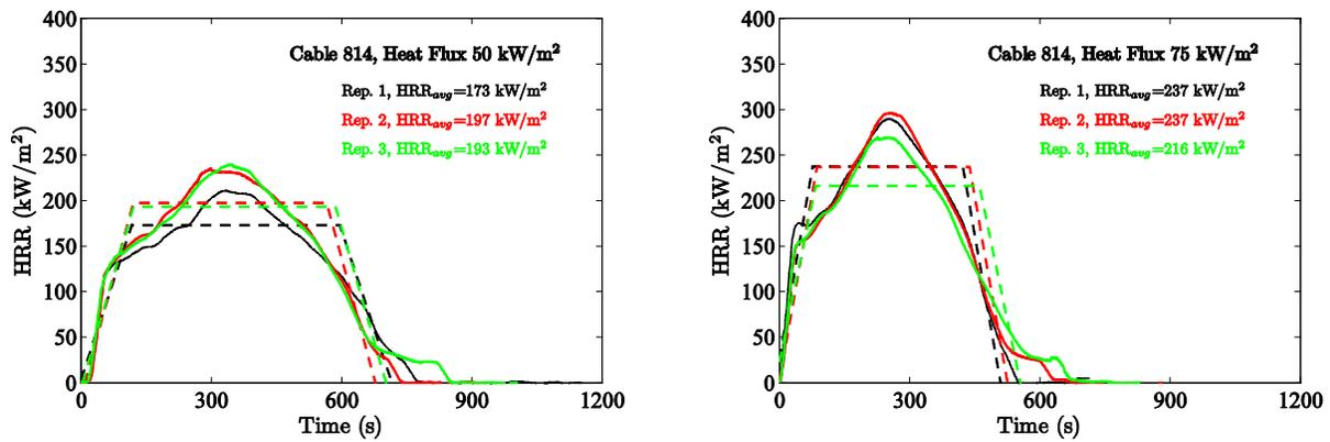
Figure 4-34. Results of cone calorimeter experiments, Cable 814.
