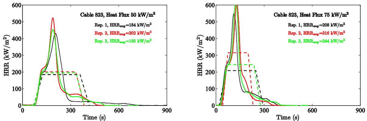
Figure 4-49. Results of cone calorimeter experiments, Cable 823.
