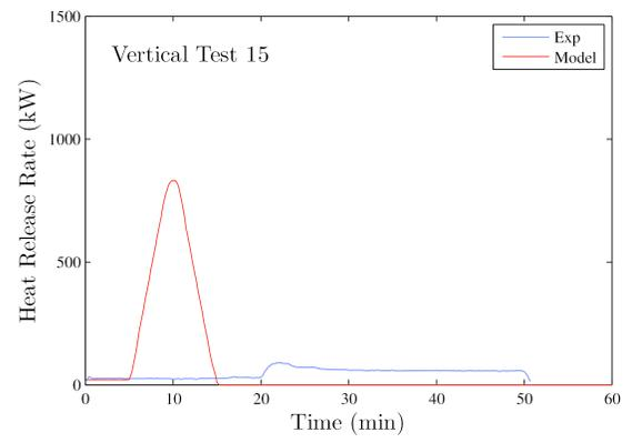
**Figure 7-3. FLASH-CAT model predictions, Vertical Tray Tests.**
