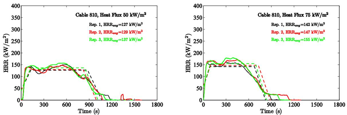
Figure 4-26. Results of cone calorimeter experiments, Cable 810.
