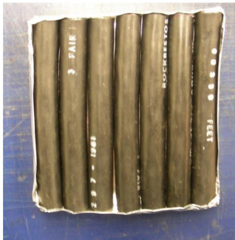
**Figure 4-1. Typical cable sample for cone calorimeter.**
