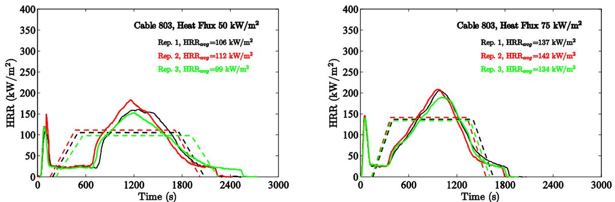
Figure 4-12. Results of cone calorimeter experiments, Cable 803.
