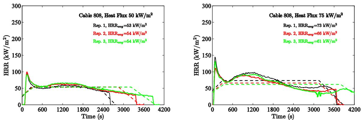
Figure 4-22. Results of cone calorimeter experiments, Cable 808.
