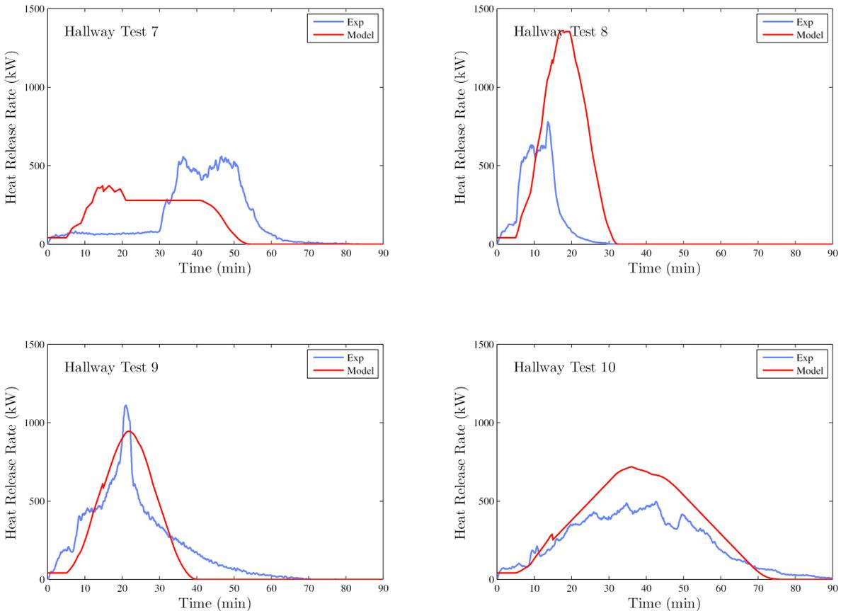
**Figure 7-2. FLASH-CAT model predictions, Corridor Tests 7-10.**
