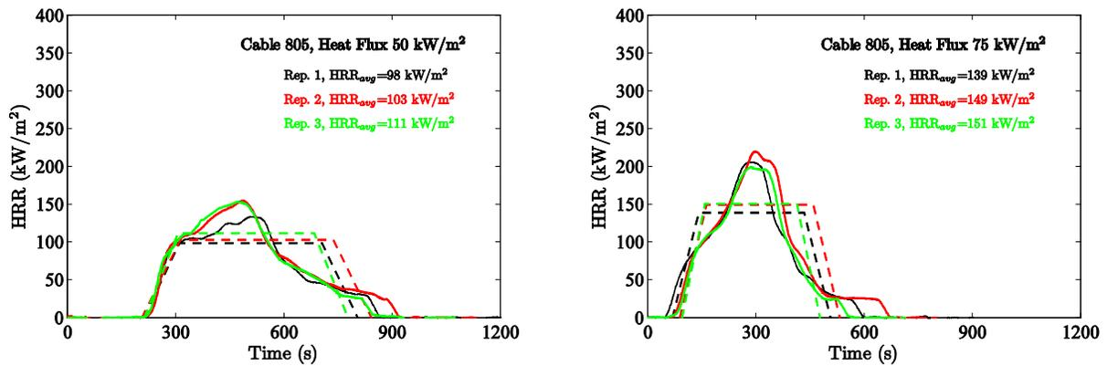
Figure 4-16. Results of cone calorimeter experiments, Cable 805.
