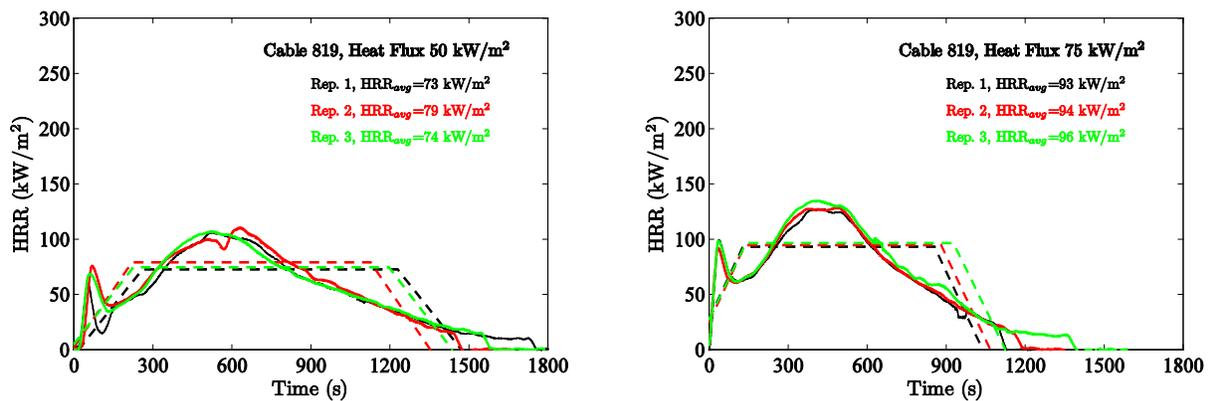
Figure 4-44. Results of cone calorimeter experiments, Cable 819.
