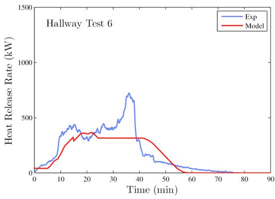
**Figure 7-1. FLASH-CAT model predictions, Corridor Tests 1-6.**
