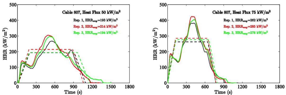
Figure 4-20. Results of cone calorimeter experiments, Cable 807.
