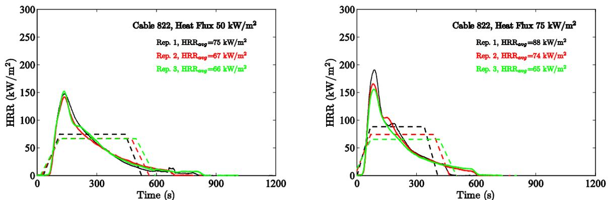
Figure 4-47. Results of cone calorimeter experiments, Cable 822.
