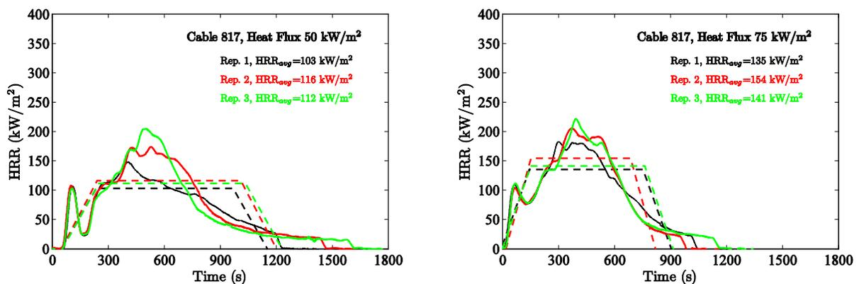
Figure 4-40. Results of cone calorimeter experiments, Cable 817.
