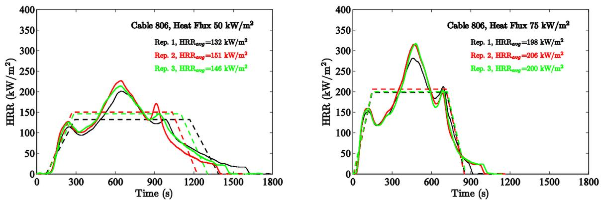
Figure 4-18. Results of cone calorimeter experiments, Cable 806.
