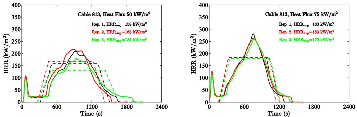
Figure 4-32. Results of cone calorimeter experiments, Cable 813.
