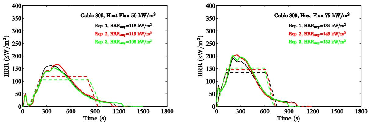
Figure 4-24. Results of cone calorimeter experiments, Cable 809.
