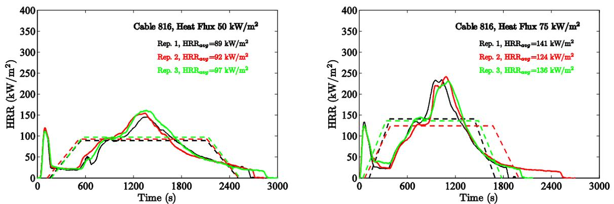
Figure 4-38. Results of cone calorimeter experiments, Cable 816.
