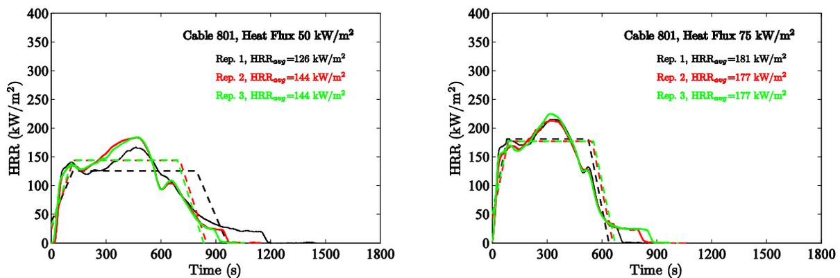
Figure 4-8. Results of cone calorimeter experiments, Cable 801.
