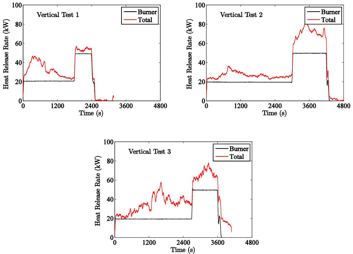
Figure 5-3. Heat release rates for Vertical Tests VT-1, VT-2, and VT-3.
