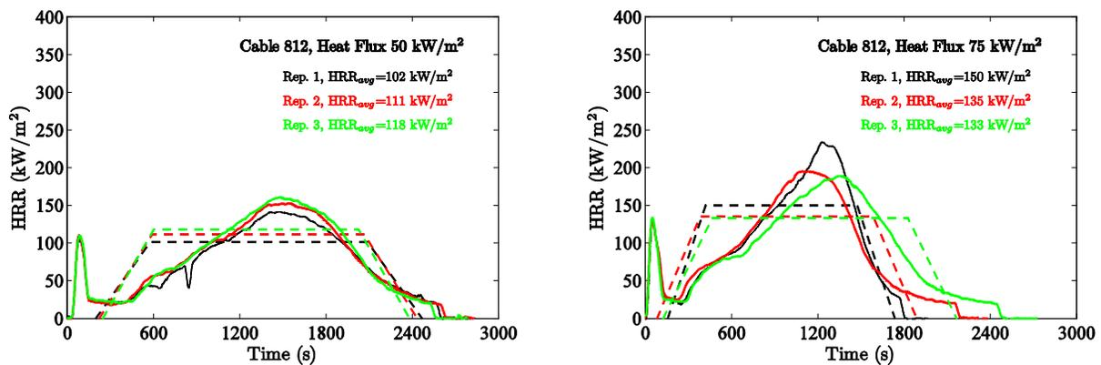
Figure 4-30. Results of cone calorimeter experiments, Cable 812.
