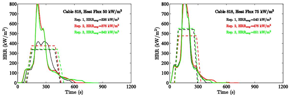
Figure 4-42. Results of cone calorimeter experiments, Cable 818.
