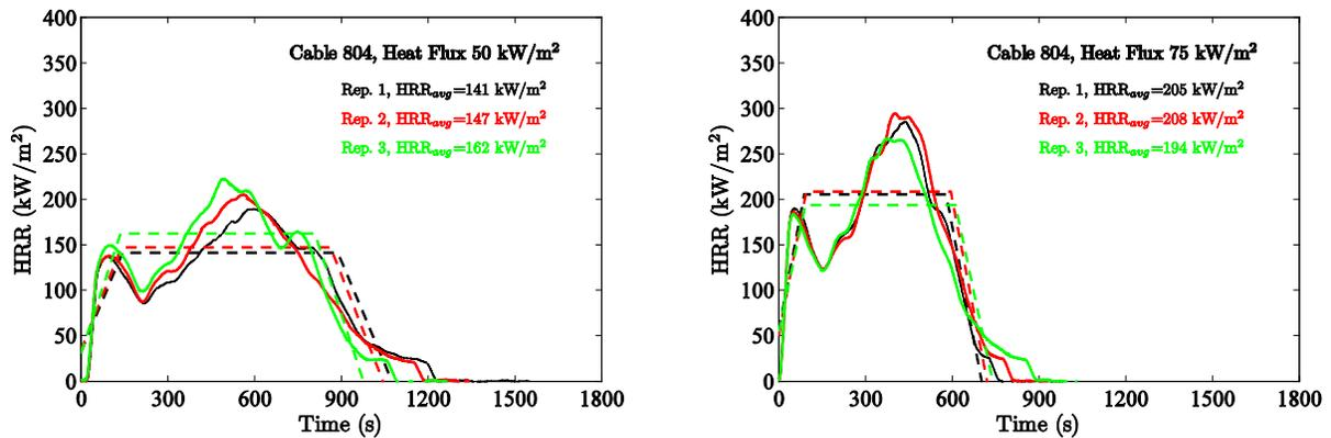
Figure 4-14. Results of cone calorimeter experiments, Cable 804.
