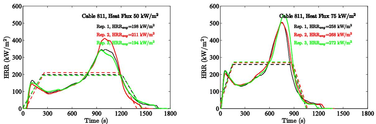
Figure 4-28. Results of cone calorimeter experiments, Cable 811.
