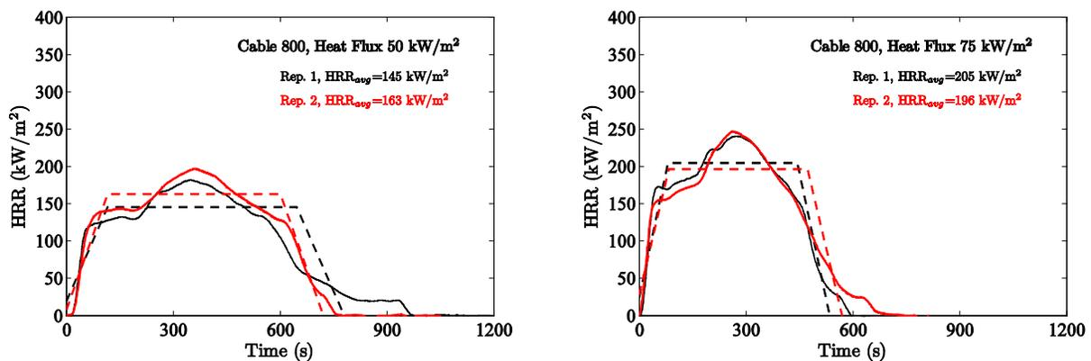
Figure 4-6. Results of cone calorimeter experiments, Cable 800.
