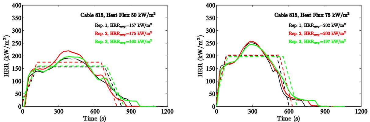
Figure 4-36. Results of cone calorimeter experiments, Cable 815.
