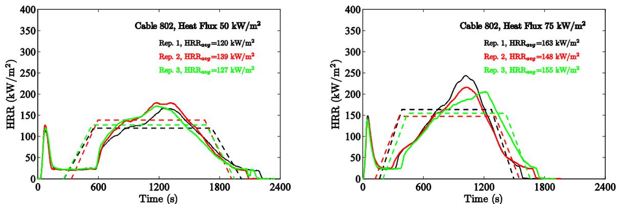
Figure 4-10. Results of cone calorimeter experiments, Cable 802.
