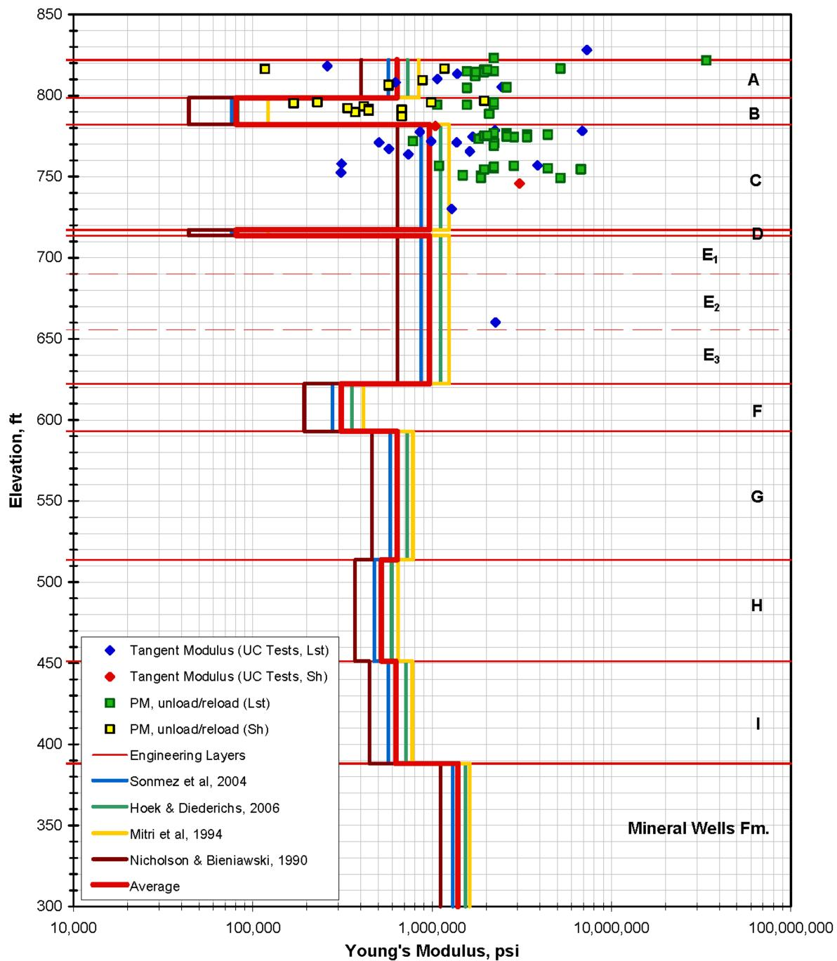
**Figure 2.5.4-245 Estimated Range of Rock Mass Modulus ( $E_{rm}$ )**
