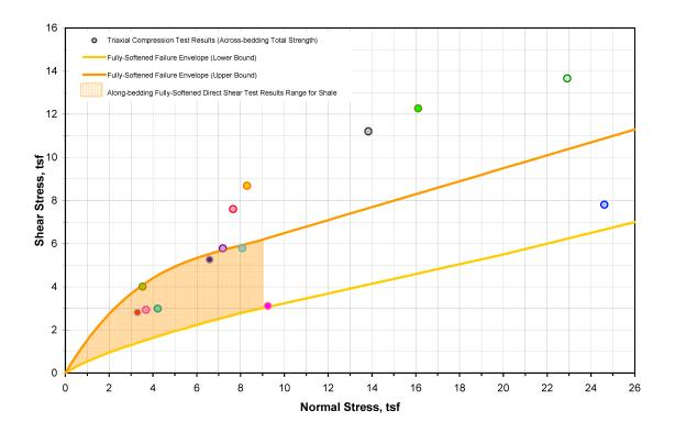
Figure 2.5.4-236 Fully-Softened Direct Shear Test Range with Triaxial Test Data
