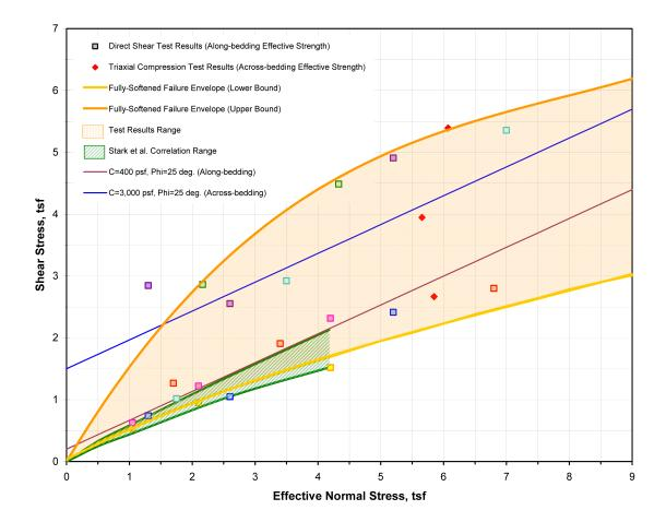
Figure 2.5.4-235 Fully-Softened Drained Shear Strength of Shale from Direct Shear and Triaxial Consolidated-Undrained Tests
