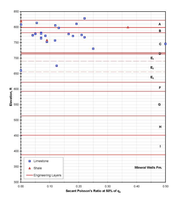
Figure 2.5.4-231 Secant Poisson's Ratio from Unconfined Compression Tests vs. Elevation
