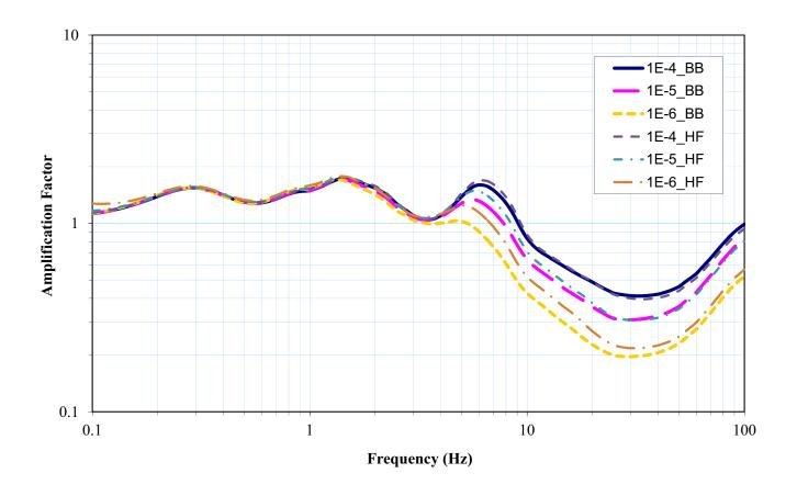
Figure 2.5.2-260 Comparison of Median Amplification Factors for the FIRS4\_SCSR (PBSRS for FIRS4) Profile: HF and BB Inputs
