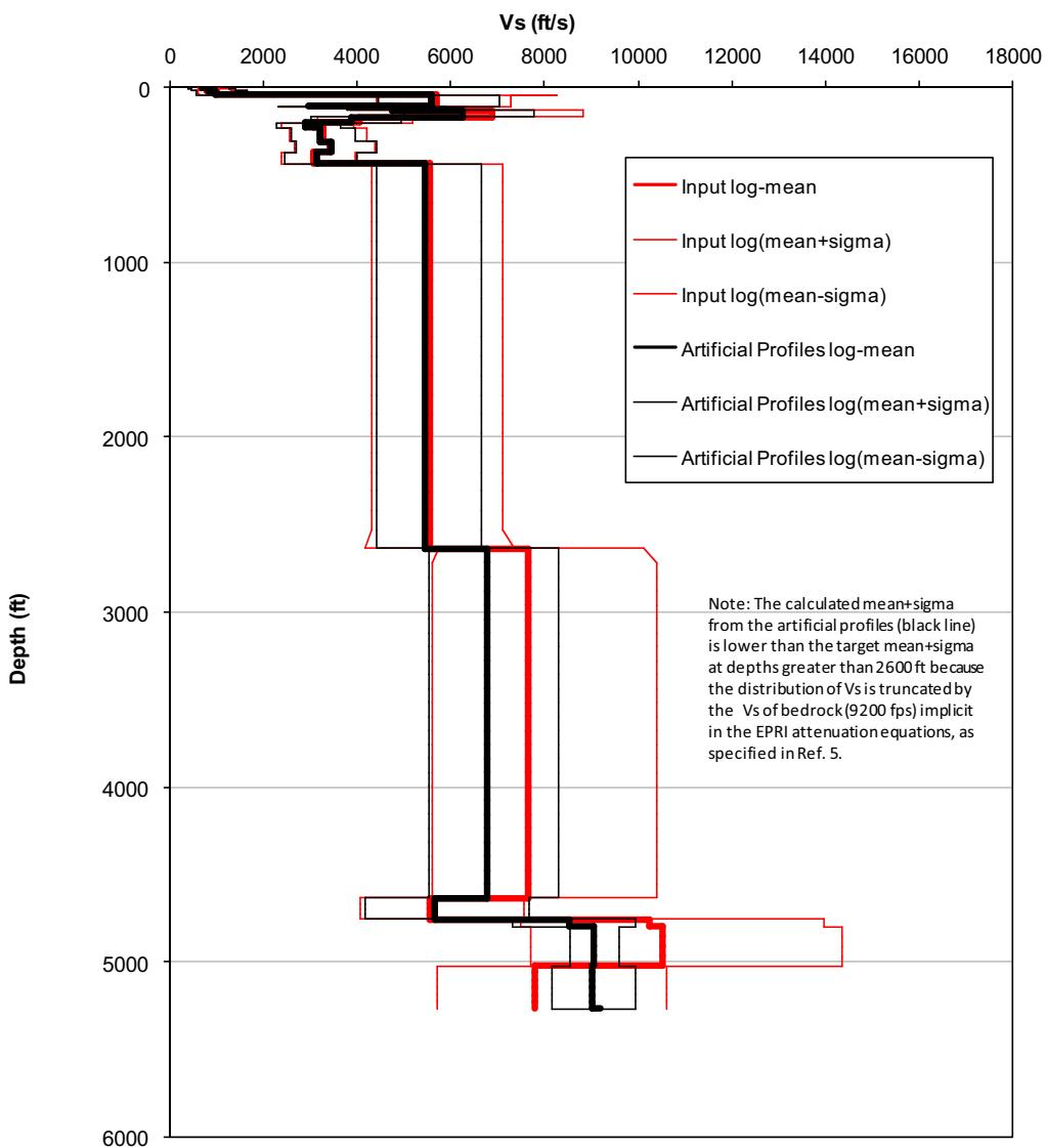
**Figure 2.5.2-237 Summary of Statistics of Synthetic Profiles Generated for the FIRS3\_COV50 Site Column**
