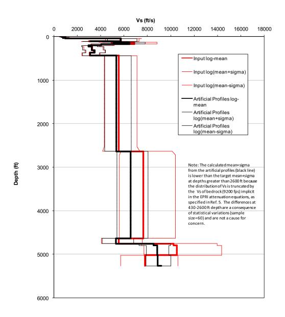
Figure 2.5.2-235 Summary of Statistics of Synthetic Profiles Generated for the FIRS3 Site Column
