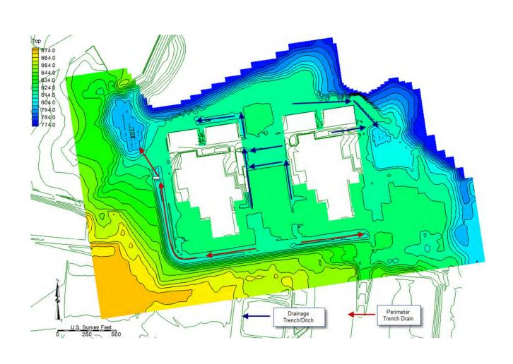
Figure 2.4.12-218 Post-Construction Surface Topography
