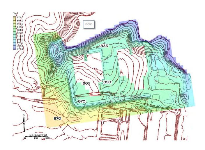
Figure 2.4.12-215 Comparison of Pre-Construction and Post Construction Surface Topography in the Model Area
