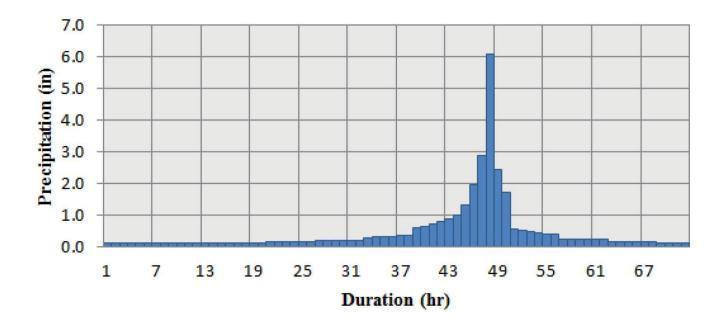
Figure 2.4.3-220 Overall Watershed, Basin 2, Two-Thirds Temporal Distribution Hyetograph (Storm Center at PR 10)
