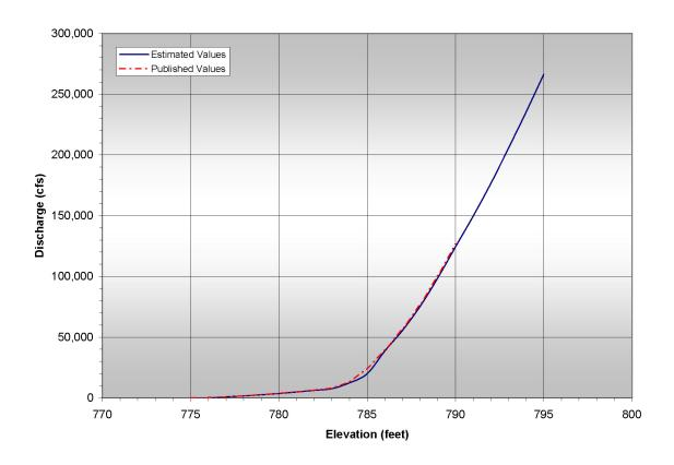
Figure 2.4.3-218 Discharge-Elevation Rating Curve
