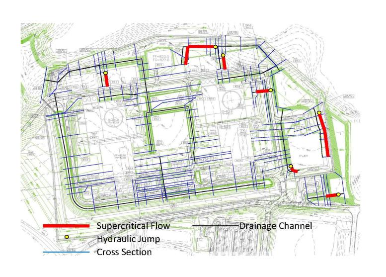
Figure 2.4.2-207 CPNPP Units 3 and 4 - Supercritical Flow & Hydraulic Jump Locations
