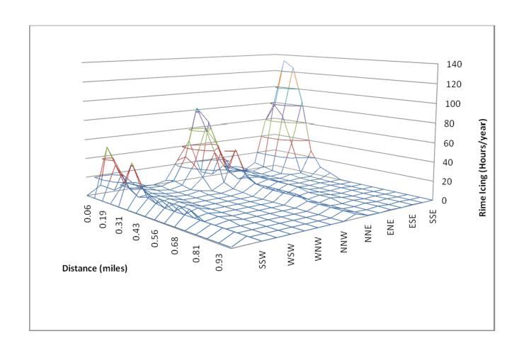
Figure 2.3-378 CPNPP Cooling Tower Annual Hours per Year Rime Icing
