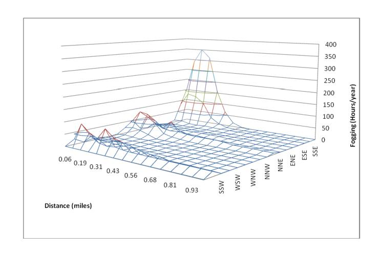
Figure 2.3-377 CPNPP Cooling Tower Annual Hours per Year Fogging
