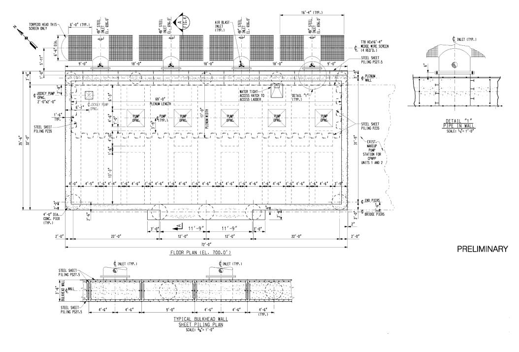
Figure 3.4-4 Makeup Water Intake Structure Floor Plan
