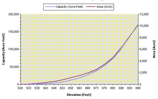
Figure 2.3-15 Lake Granbury Elevation - Area - Capacity Curve
