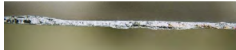
Boraflex edge showing oxidation and delamination EPRI TR-1013721
