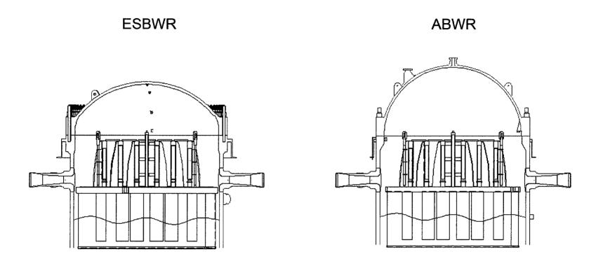
Figure 2.1-1. Comparison of Planned ESBWR and Typical ABWR Vessel Steam Regions
