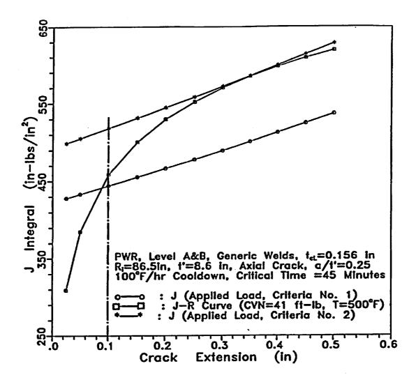
Figure A-3: Acceptable Upper-Shelf Energy in a PWR Vessel for Service Levels A and B.
