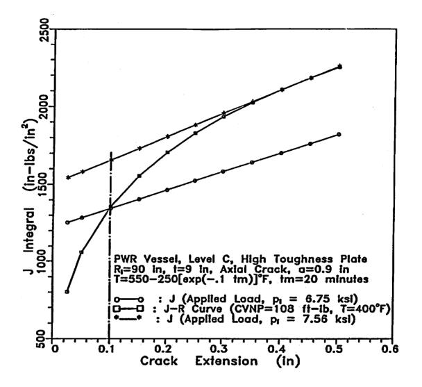
Figure A-4: Safety Margin Evaluation in a PWR Vessel for Service Level C.
