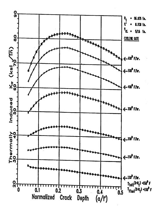
Figure A-6: Peak Thermal Stress Intensity Factors in a PWR Vessel for Transients with Several Different, but Constant, Cooldown Rates.
