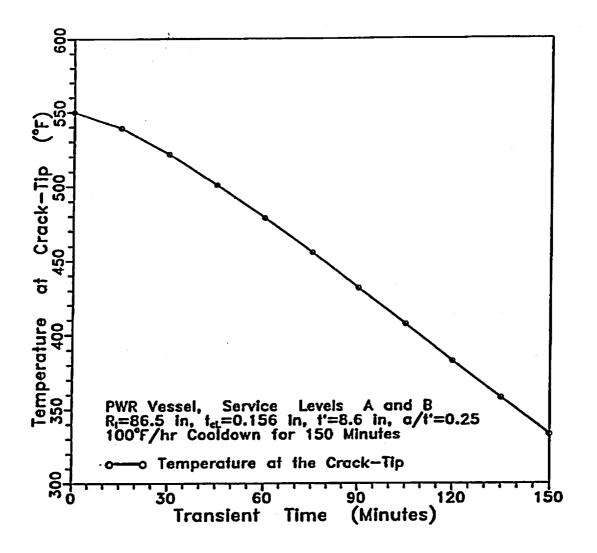
Figure A-1: Transient Temperature History at Crack Tip for Service Levels A and B.
