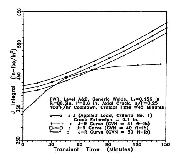
Figure A-2: J-Applied and J-R Curve History at Crack Tip for Service Levels A and B at a Crack Extension of 0.1 inch.
