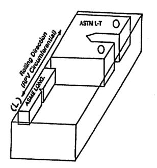
Figure 2. Definition of the ASME and ASTM Flaw Orientations in an RPV.
