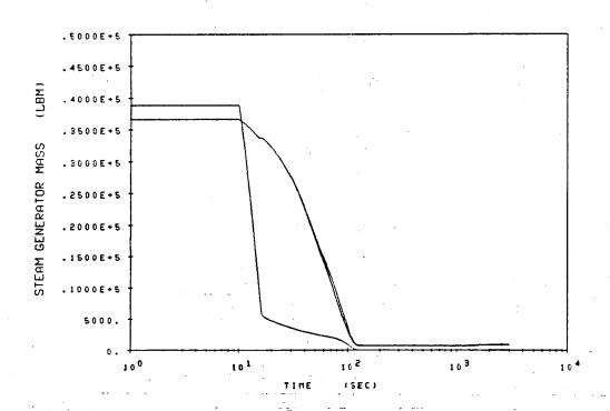
Case 5 - Downstream Break 103% power 175gpm AFW at 20 minutes
