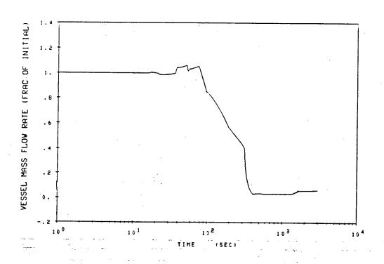
Case 🖹 - Downstream Break 103% power 175gpm AFW at 20 minutes
