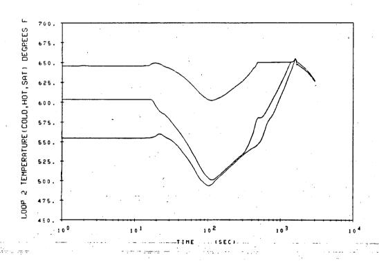
Case &F - Downstream Break 103% power 175gpm AFW at 20 minutes
