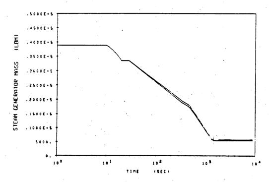
FIGURE 4 Steam Generator Pressure and Steam Generator Mass vs. Time Case  $\frac{D}{2}$ : SONGS 1 FLB Upstream of In-Containment Check Valves at 100% Power AFW = 100 gpm to 2 steam generators at 30 minutes
