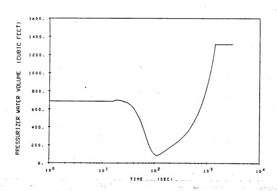
Case 5 - Downstream Break 103% power 175gpm AFW at 20 minutes
