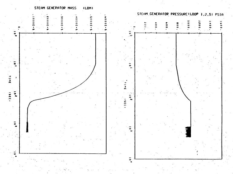
Case E: SONGS 1 FLB Upstream of In-Containment Check Valves at 50% Power AFW = 100 gpm to 2 steam generators at 15 minutes
