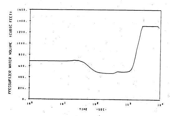
FIGURE 2 Pressurizer Pressure and Pressurizer Water Volume vs. Time
