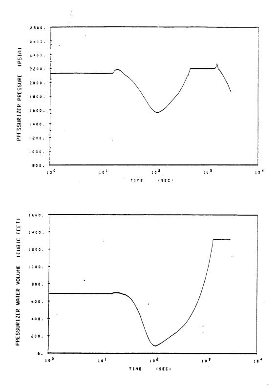
San Onofre Nuclear Generating Station Unit 1 - Feedline Break Case F - Downstream Break 103% power 175gpm AFW at 20 minutes
