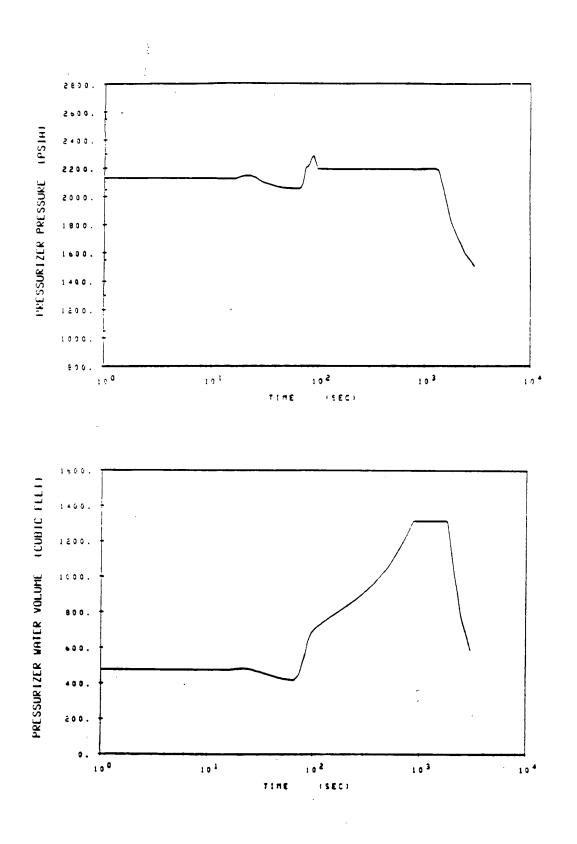
San Onofre Nuclear Generating Station Unit 1 - Feedline Break Case G - Downstream Break 53% power 175gpm AFW at 15 minutes Pressurizer Pressure & Water Volume vs. Time
