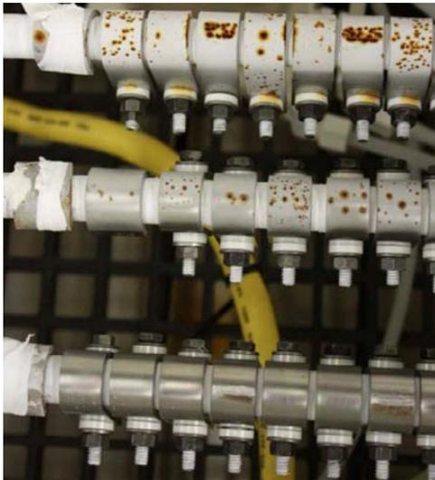
Pitting on specimens at 10 g/m<sup>2</sup> (top), 1 g/m<sup>2</sup> (middle), and 0.1 g/m<sup>2</sup> (bottom)
