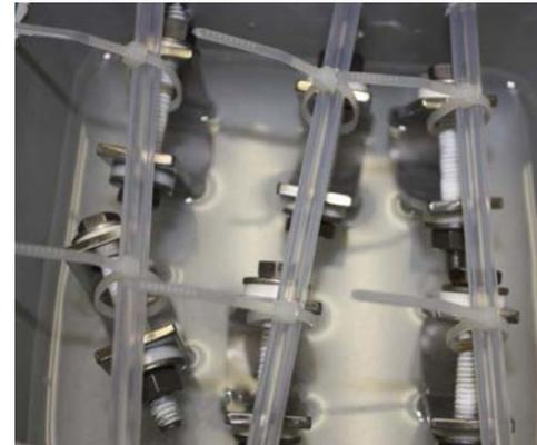
U-bend specimens immersed in solution
