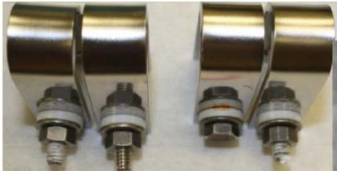
Specimens immersed in sea salt after 5 weeks, as received (L); sensitized (R)
