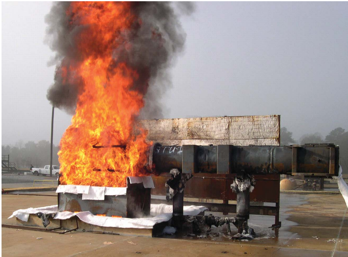
Figure 3-19 December 15, Impact Limiter Burn Test
