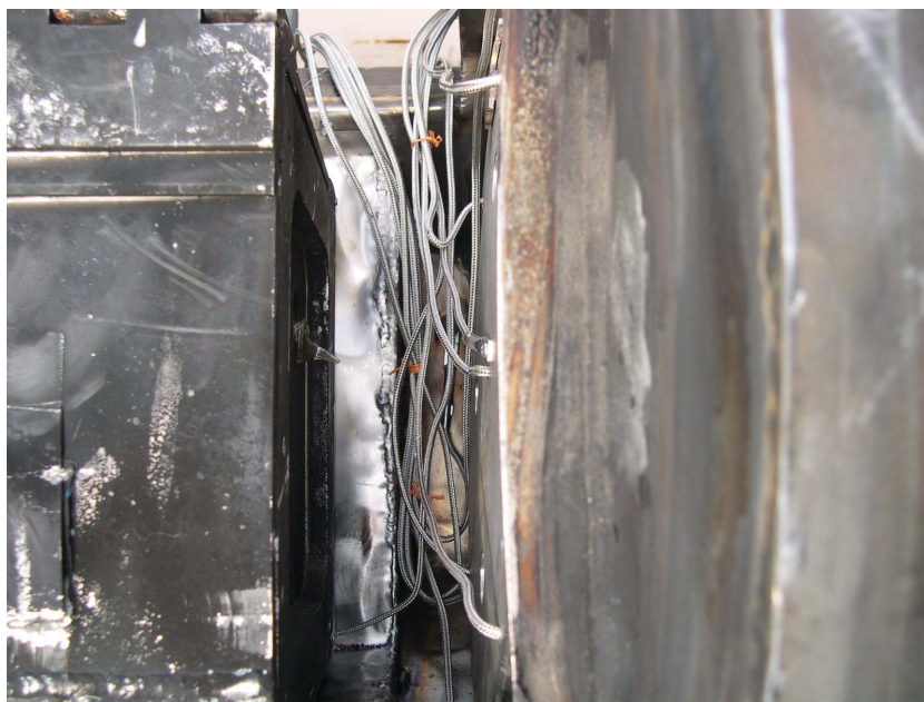
Figure 3-23 Outerpack Internals after December 15 Burn Test
