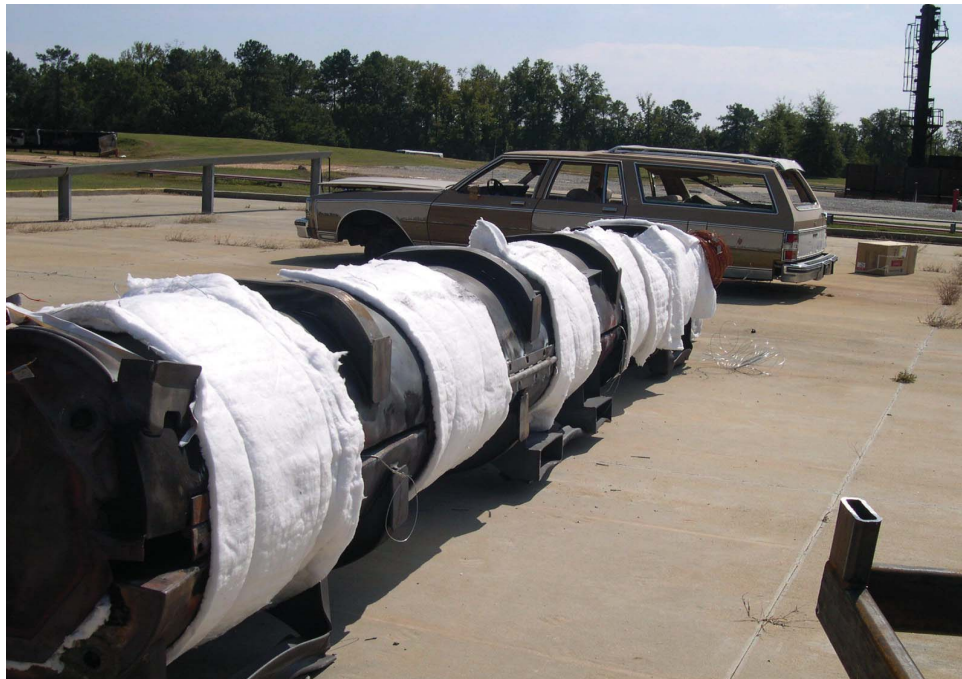
Figure 3-11 Package Exterior Wrapped with Ceramic Fiber Insulation
