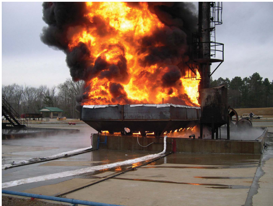
Figure 3-4 December 15, Impact Limiter Burn Test
