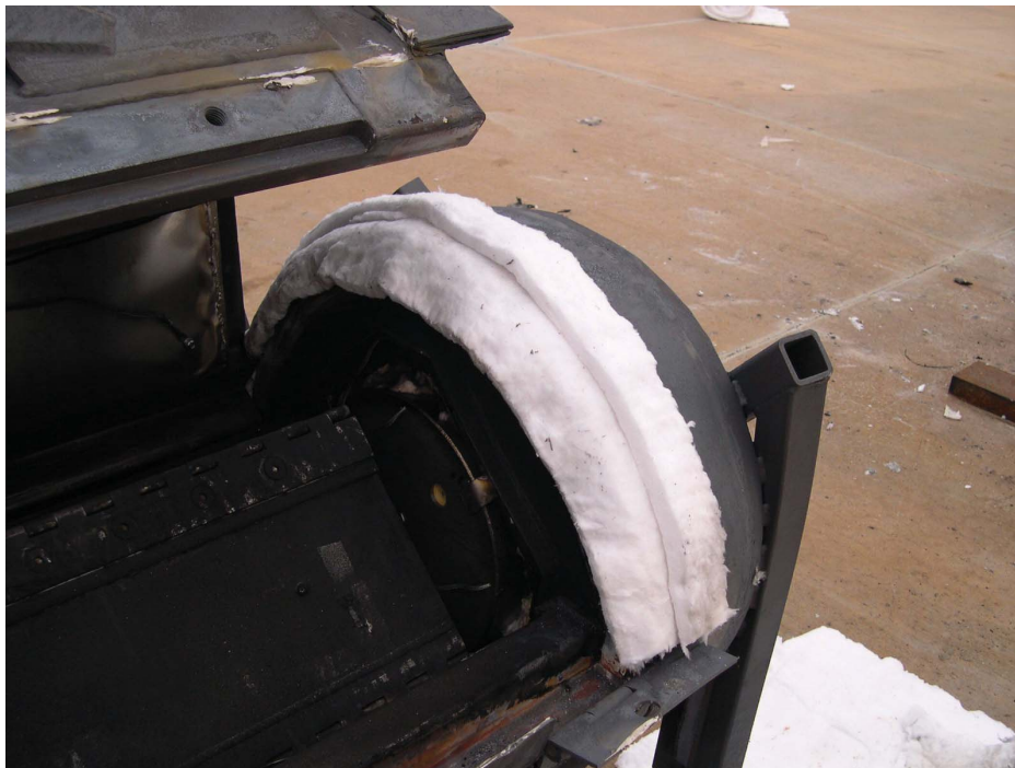
Figure 3-24 Kaowool Layers on Outerpack Bottom Impact Limiter
