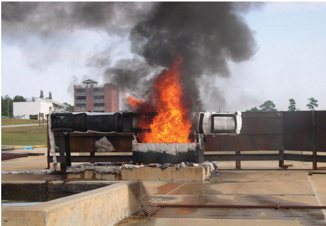
Figure 3-3 Seam Burn Test
