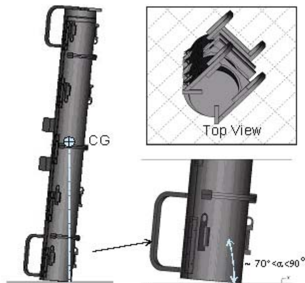
Figure 2-43 Top Nozzle Analysis Drop Orientation
