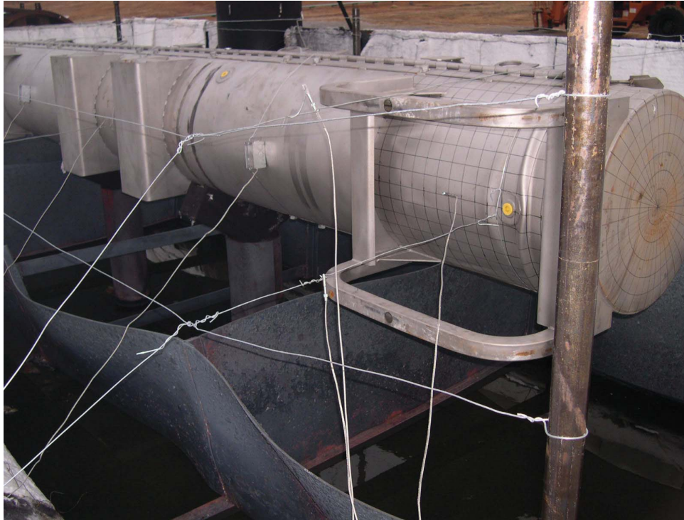
Figure 3-32 Test Stand for Fire Test
