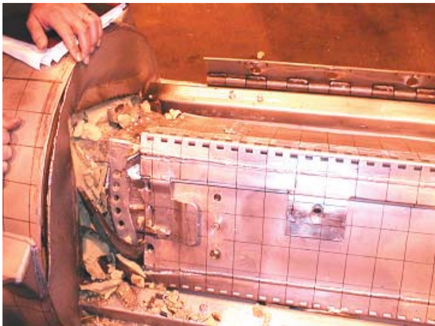
Figure 2-128 Traveller Prototype Clamshell and Bottom Impact Limiter After Test Series 3
