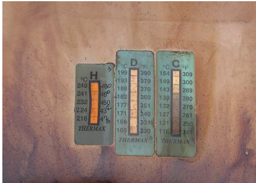
Figure 3-8 Temperature Strip Condition After CTU Burn Test
