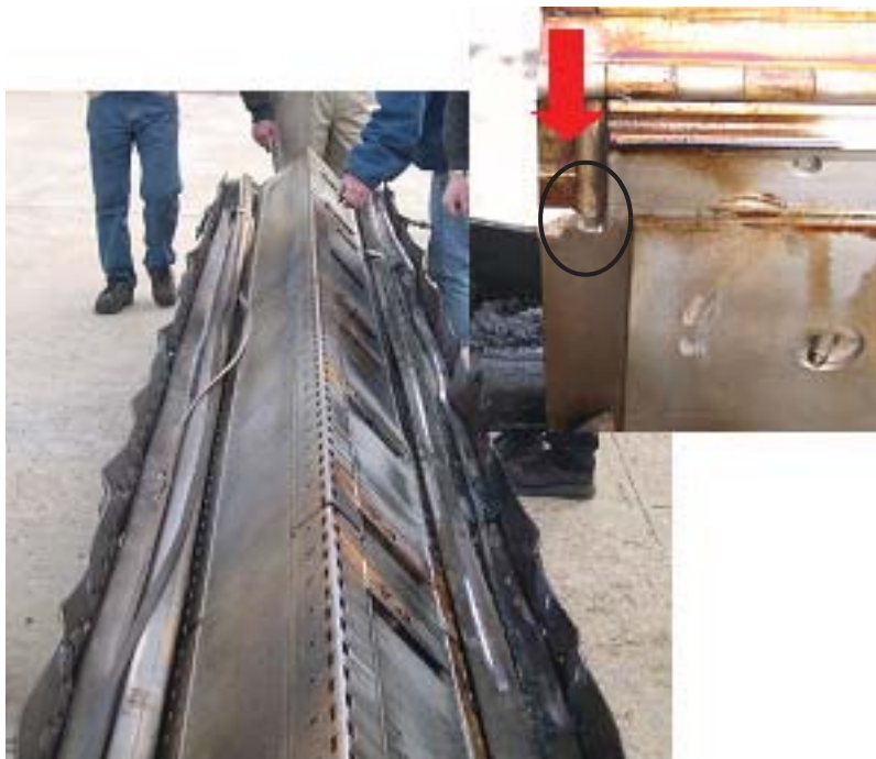
Figure 2-149 CTU Clamshell After Drop and Fire Tests
