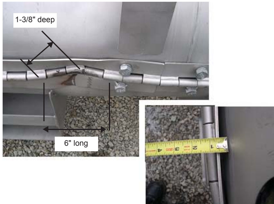
Figure 2-148 CTU Outerpack After Test 3
