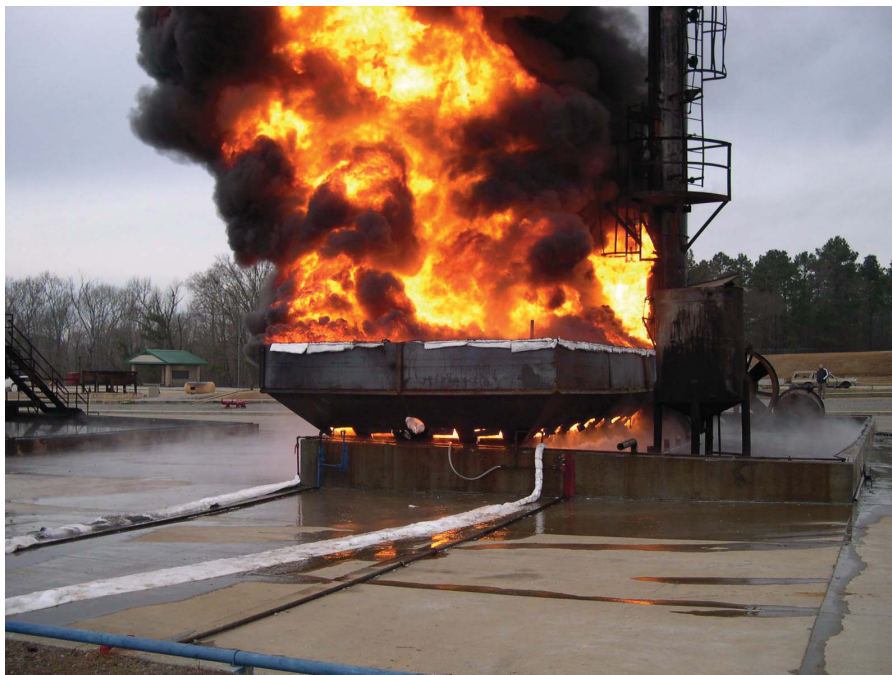
Figure 3-6 Traveller CTU During Pool Fire Test
