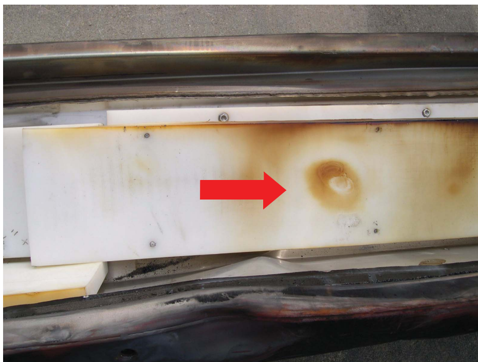
Figure 3-44 Localized Melt Spot in Lid Moderator Block
