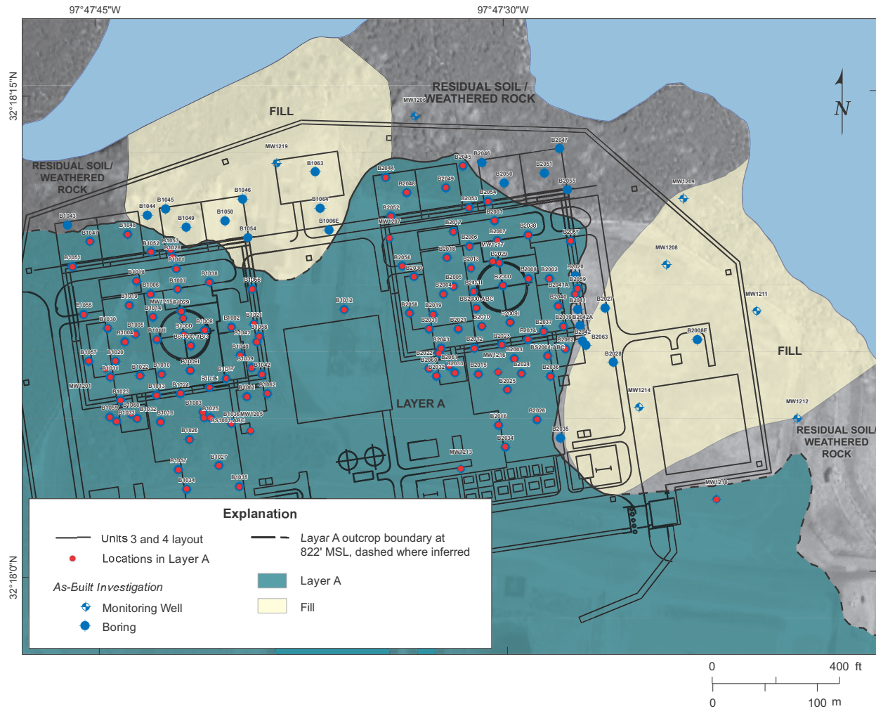
Figure 2.5.4-215 Plant Grade Outcrop Map at Elevation 822 ft
