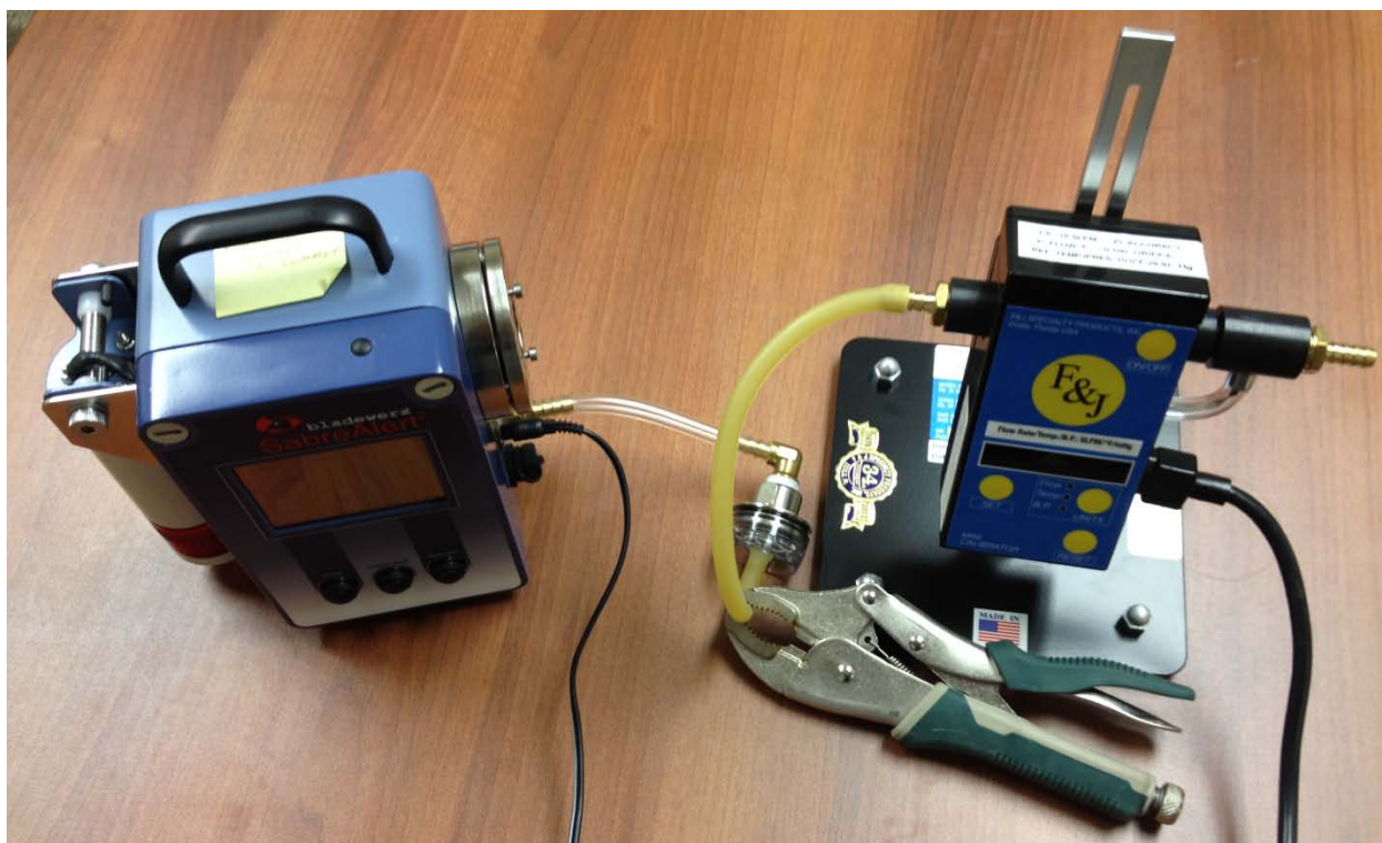
Figure 1 Flow Calibration Setup
