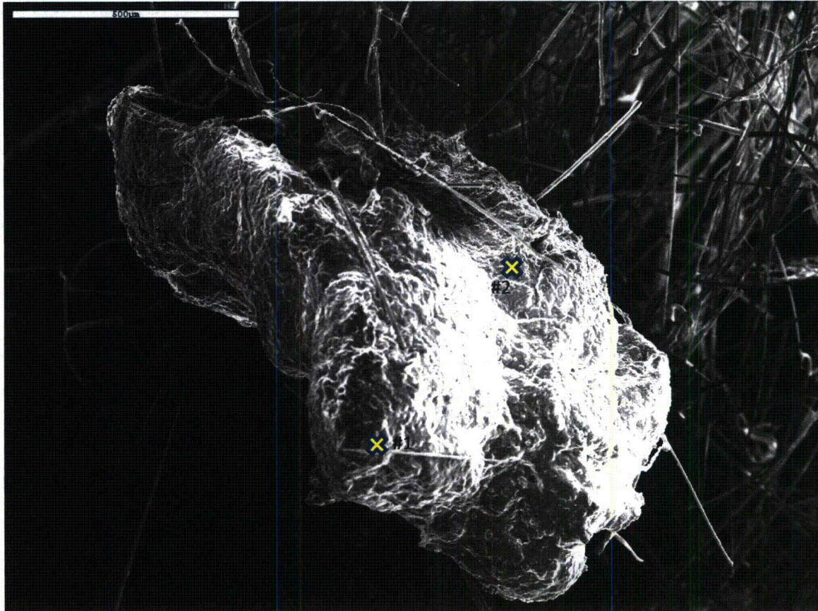
Figure 59 - "NEI, white flakes, 1" Layered particle on fiber
